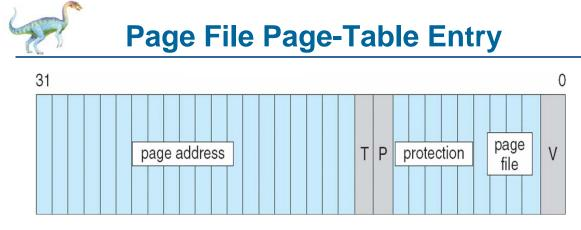
5 bits for page protection, 20 bits for page frame address, 4 bits to select a paging file, and 3 bits that describe the page state. V = 0
