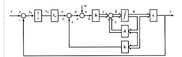
An internal model control configuration with state feedback
