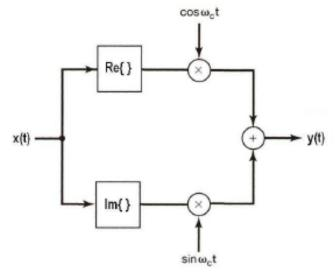
real part and imaginary part of the input, respectively. Find an expression for the Fourier transform  $Y(j\omega)$  of the output signal y(t). Plot the real and imaginary parts of  $Y(j\omega)$ .
