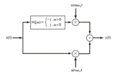
Assume that the message signal x(t) has its spectrum  $X(j\omega) = 0$  for  $|\omega| > \omega_M$  and  $\omega_c > \omega_M$ .
