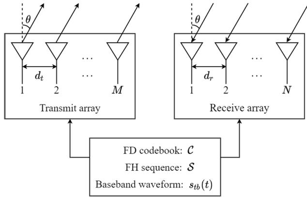
FIGURE 2. Configuration of co-located FH-LFM-FD-MIMO radar.
