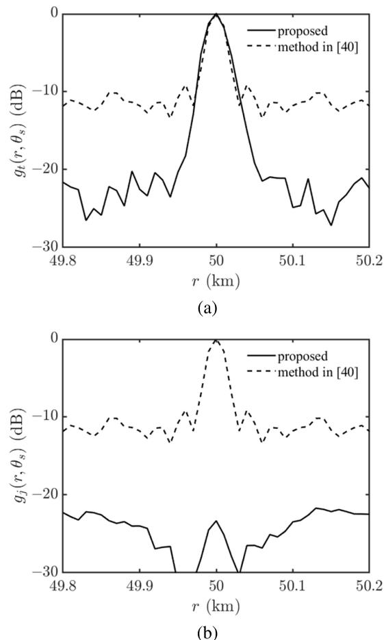
**FIGURE 15.** Range profiles of (a) average normalized response defined in (51) and (b) average response to jamming signals defined in (52), at  $\theta_s = 0^\circ$ .
