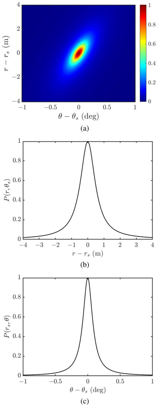
**FIGURE 16.** MVDR spectrum in target range-azimuth cell, centered at  $r_s = 50$  km,  $\theta_s = 0^\circ$ , (a) two-dimensional spectrum, (b) spectrum at  $\theta_s = 0^\circ$ , (c) spectrum at  $r_s = 50$  km, SNR = 10 dB.
