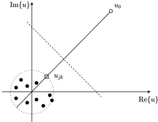
**FIGURE 7.** Target detection in  $u$  plane,  $\circ$ : target echo,  $\bullet$ : jamming signals,  $\square$ : strongest jamming signal,  $- - -$ : boundary line (threshold) when  $\bar{\eta}_0 = \bar{c}_k \in \mathcal{C}$ .
