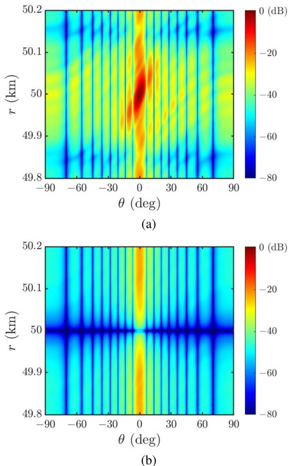
**FIGURE 14.** Range-azimuth profiles of (a) average normalized response defined in (51) and (b) average response to jamming signals defined in (52).
