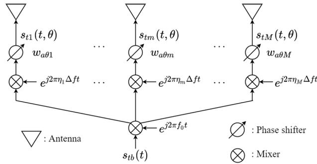
FIGURE 3. Schematic of transmit array.
