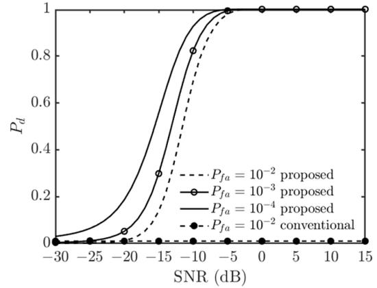
FIGURE 9. Average detection probability  $P_d$  versus SNR at different  $P_{fa}$ 's, conventional radar without FH scheme is shown for comparison.
