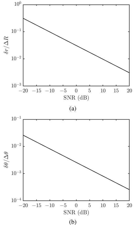
**FIGURE 17.** Ratio of (a)  $\delta r / \Delta r$  and (b)  $\delta \theta / \Delta \theta$  versus SNR.
