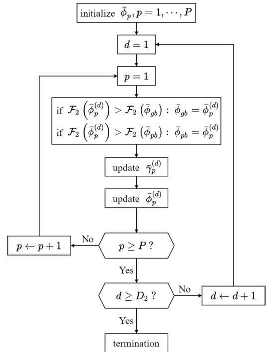
FIGURE 6. Flow-chart of optimizing spotlight-range beamforming vector.
