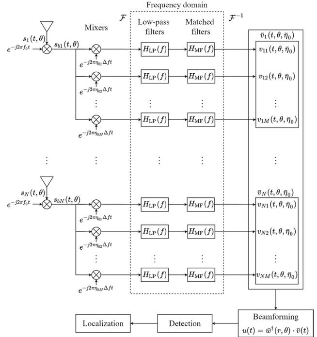
FIGURE 4. Schematic of receive array.
