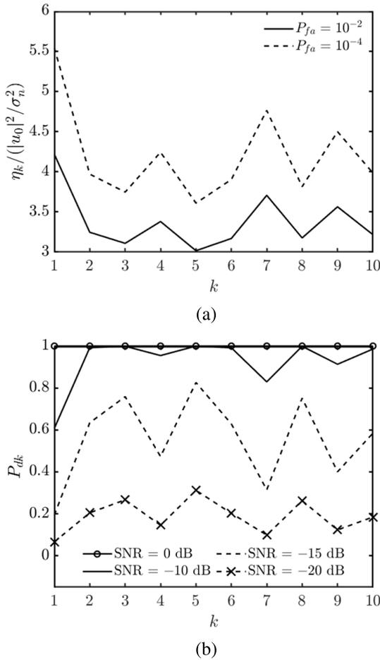
FIGURE 8. (a) Normalized threshold,  $\eta_k / (|u_0|^2 / \sigma_n^2)$ , versus FD code index  $k$  at different  $P_{fa}$ 's, SNR = 10 dB. (b)  $P_{dk}$  versus FD code index  $k$ ,  $P_{fa} = 10^{-2}$ , at different SNRs.
