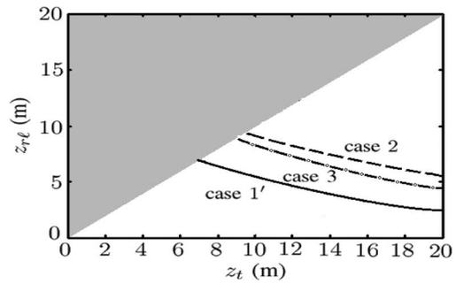
Fig. 6. Lowest receiving height ( $z_{rl}$ ) versus transmitting antenna height ( $z_t$ ) with  $\delta_{PF} = 0.2$  dB. (Solid line) Case 1',  $F = 0.25$  m,  $D = 1$  m, and  $x_r = 1.5$  km. (Dash line) Case 2. (Dash-dotted line) Case 3.
