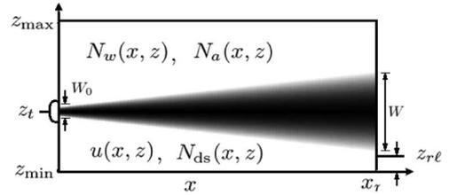
Fig. 2. Schematic of millimeter-wave propagation in an SDS.
