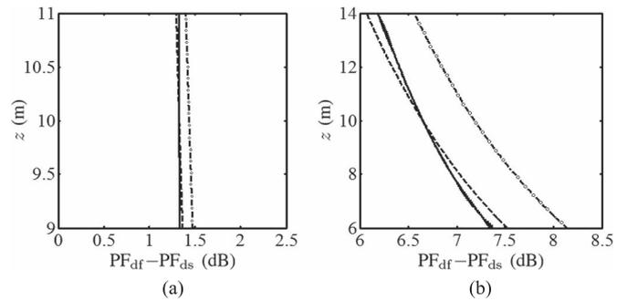
Fig. 7. Height profile of  $PF_{df} - PF_{ds}$  in case 3 (a) at  $x_r = 0.1$  km and (b) at  $x_r = 0.5$  km. (Solid line) PWE method. (Dash line) Formula in [10]. (Dash-dotted line) Formula in [13].
