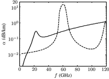
Fig. 3. Specific attenuation attributed to (dash line) dry air [18] and (solid line) water vapor [18].
