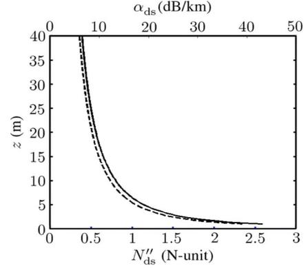
Fig. 1. Height profiles of (solid line) specific attenuation constant  $\alpha_{ds}$  and (dash line)  $N''_{ds}$ ;  $f = 100$  GHz,  $N_{ts} = 5 \times 10^7$ , and  $\epsilon_d = 3.5 - j1.64$  [10].
