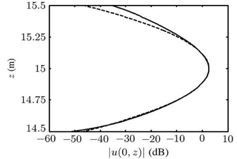
Fig. 4. Magnitude of the aperture field on the transmitting antenna. (Solid line) Parabolic reflector with feeding horn;  $D = 1.2$  m and  $F = 0.3$  m. (Dash line) Gaussian beam with  $W_0 = 0.22$  m.
