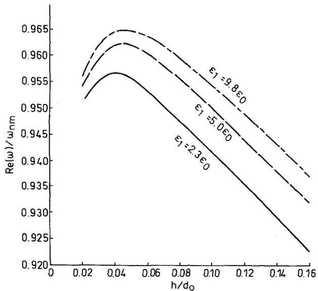
**Fig. 5** Real part of (0,1) mode resonant frequency of wraparound patch with two-lamina G/E composite ground plane
