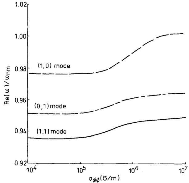
**Fig. 6** Real part of resonant frequency of wraparound patch with two-lamina G/E composite ground plane
