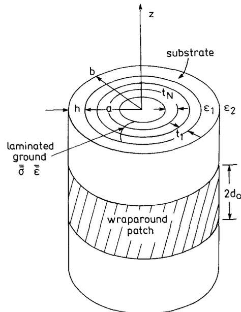
Fig. 1 Geometrical configuration of wraparound patch on laminated composite ground plane
