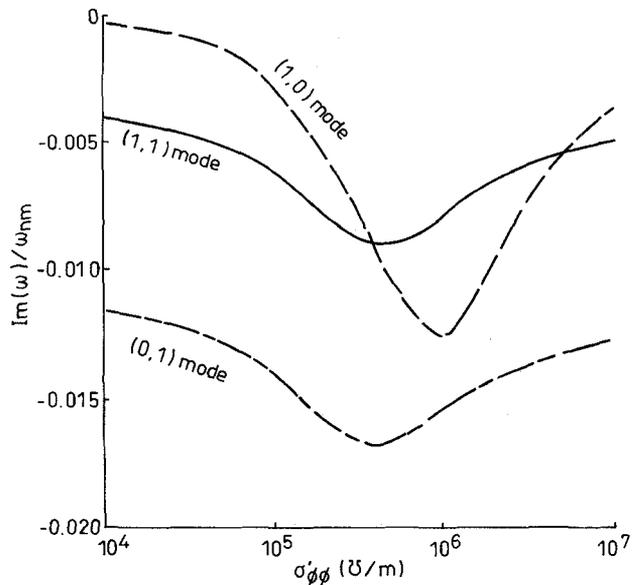
**Fig. 7** Imaginary part of resonant frequency of wraparound patch with two-lamina G/E composite ground plane
