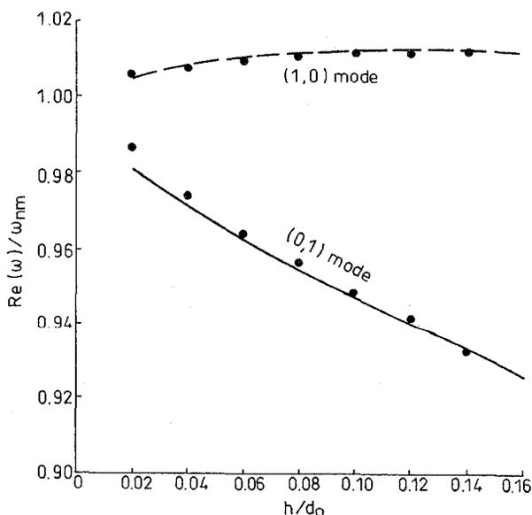
**Fig. 2** Real part of resonant frequency of wraparound patch with one lamina of solid copper ground plane
