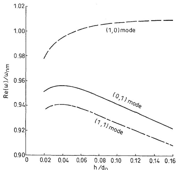
**Fig. 3** Real part of resonant frequency of wraparound patch with two-lamina G/E composite ground plane
