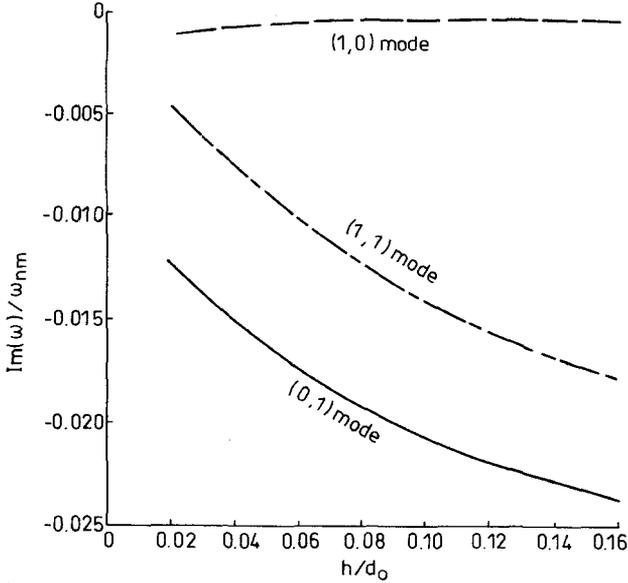
**Fig. 4** Imaginary part of resonant frequency of wraparound patch with two-lamina G/E composite ground plane
