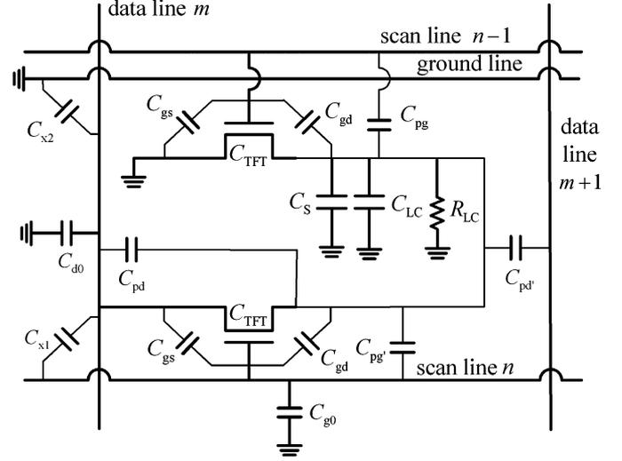
Fig. 4. Equivalent circuit of a DTFT subpixel.
