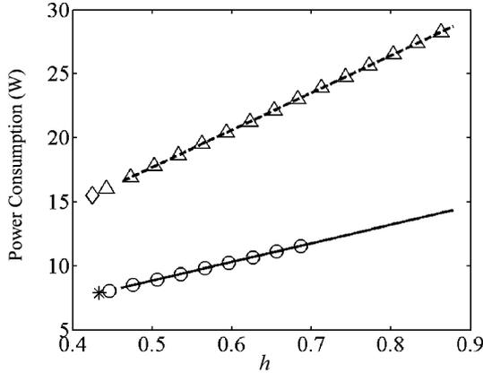
Fig. 10. Power consumption of 30'' WXGA LCDs, \*:  $W_{30'',DTFT} = 25 \mu\text{m}$ ,  $\circ$ :  $W_{30'',DTFT} = 40 \mu\text{m}$ , —:  $W_{30'',DTFT} = 54 \mu\text{m}$ ,  $\diamond$ :  $W_{30'',STFT} = 34 \mu\text{m}$ ,  $\triangle$ :  $W_{30'',STFT} = 70 \mu\text{m}$ , - - -:  $W_{30'',STFT} = 108 \mu\text{m}$ .
