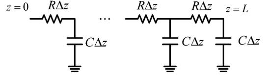
Fig. 2. Signal line modeled as a cascade of infinitesimal  $RC$  segments.
