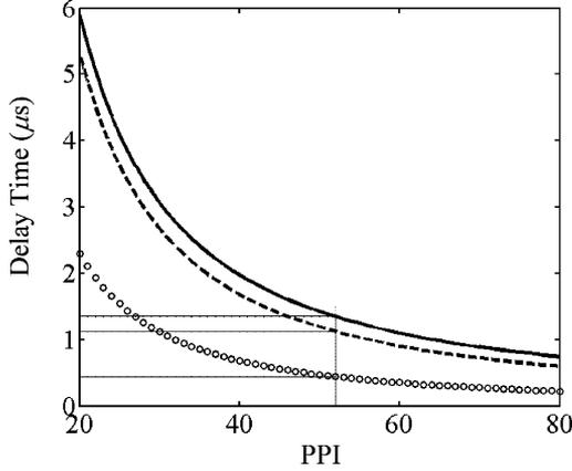
Fig. 8. Delay over signal line, —: scan-line delay of DTFT, --: scan-line delay of STFT and o: data-line delay of DTFT and STFT, PPI = 52 for 30'' WXGA.
