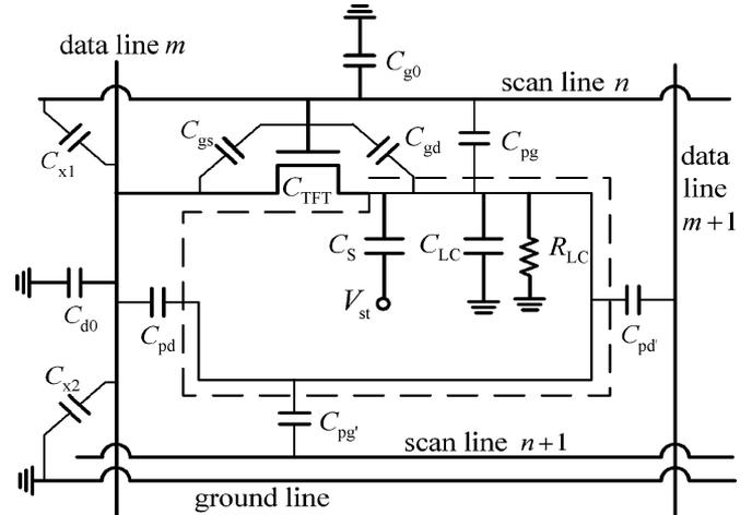
Fig. 1. Equivalent circuit of a subpixel.
