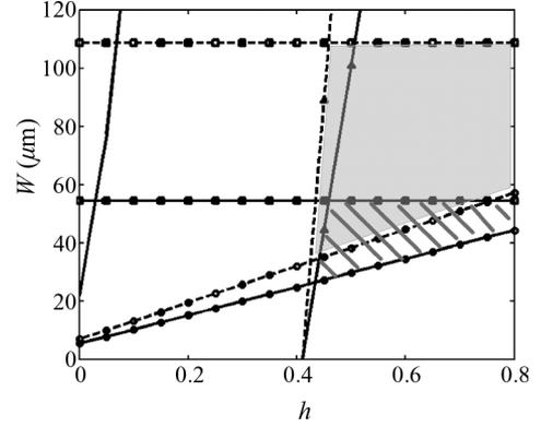
Fig. 9. Operation windows of subpixel design of 30'' WXGA LCDs, slit area with DTFT, grey area with STFT, —o—: charging (DTFT), --o--: charging (STFT), —△—: holding (DTFT), --△--: holding (STFT), —: asymmetric kickback (DTFT)(STFT), —[]—: scan-line delay (DTFT), and --[]--: scan-line delay (STFT).
