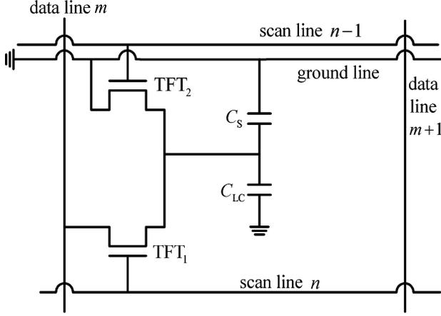
Fig. 3. Configuration of charge-recycling circuit using DTFTs.
