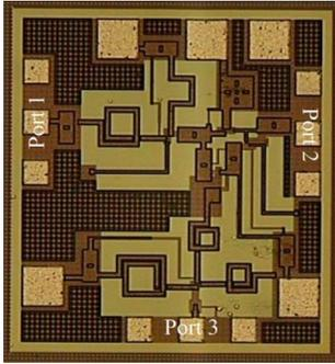
Fig. 3. Chip photo of the proposed active quasi-circulator.
