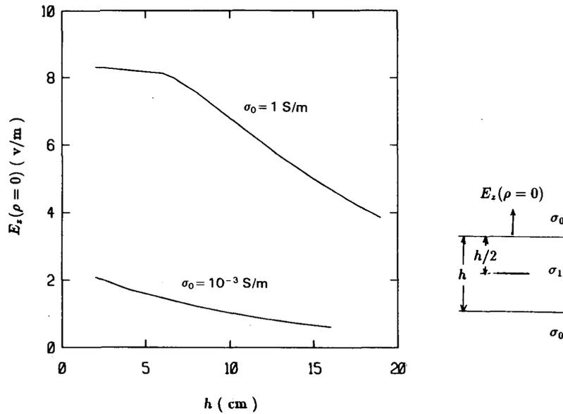
Fig. 7. Electric field at the interface of a three-layer medium,  $w_p^x = w_p^y = 10$  cm,  $w_h^x = w_h^y = 2$  cm,  $w_e^x = w_e^y = 1.6$  cm,  $V_p = V_e = 1$  V,  $\sigma_1 = 10$  S/m.
