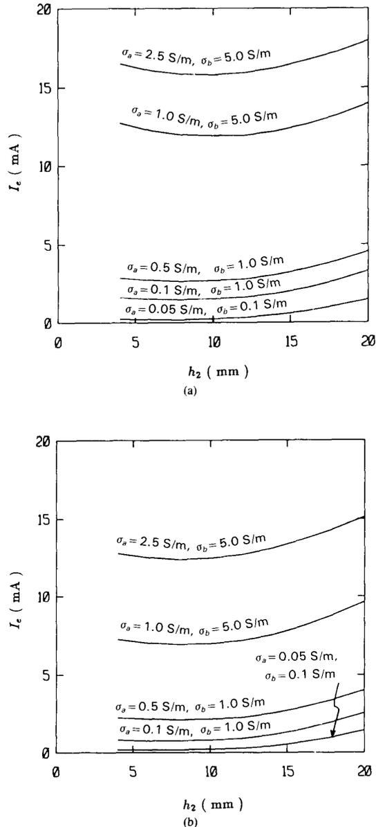
Fig. 13. (a) Total electrode current of a pad-electrode with an inversion conductivity profile ( $D = 1$  cm),  $w_p^x = w_p^y = 10$  cm,  $w_h^x = w_h^y = 2$  cm,  $w_c^x = w_c^y = 1.6$  cm,  $V_p = V_e = 1$  V,  $h_1 = 2$  cm. (b) Total electrode current of a pad-electrode with an inversion conductivity profile ( $D = 3$  cm),  $w_p^x = w_p^y = 10$  cm,  $w_h^x = w_h^y = 2$  cm,  $w_c^x = w_c^y = 1.6$  cm,  $V_p = V_e = 1$  V,  $h_1 = 2$  cm.
