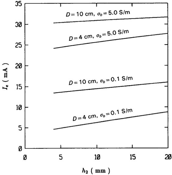
Fig. 12. Total electrode current of a pad-electrode with a parabolic conductivity profile,  $w_p^x = w_p^y = 10$  cm,  $w_h^x = w_h^y = 2$  cm,  $w_e^x = w_e^y = 1.6$  cm,  $V_p = V_e = 1$  V,  $h_1 = 2$  cm.
