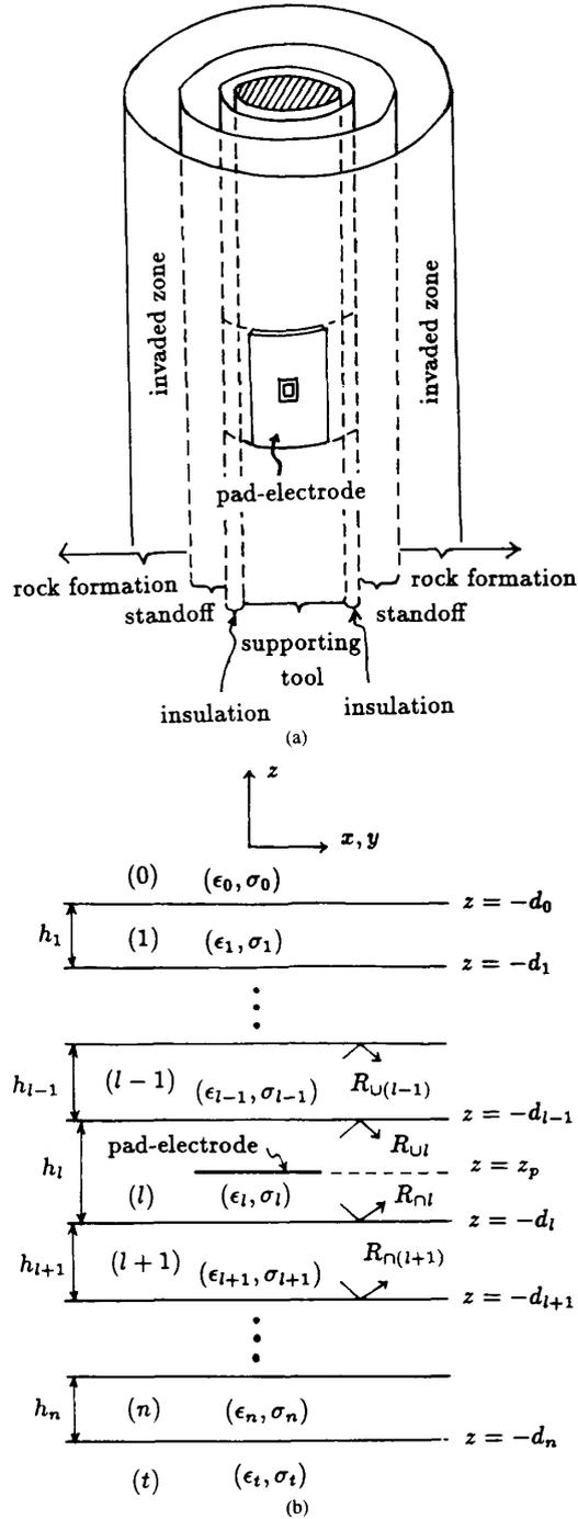
Fig. 1. (a) Geometrical configuration of a pad-electrode embedded in the borehole environment. (b) Geometrical configuration of a pad-electrode embedded in layer ( $l$ ) of a planar stratified medium.
