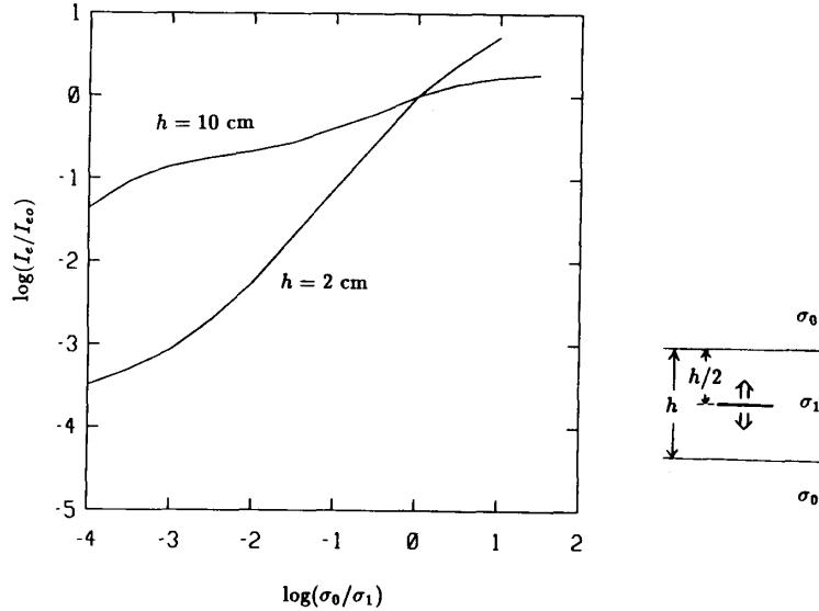
Fig. 4. Total electrode current of a pad-electrode in a three-layer medium,  $w_p^x = w_p^y = 10$  cm,  $w_h^x = w_h^y = 2$  cm,  $w_e^x = w_e^y = 1.6$  cm,  $V_p = V_e = 1$  V,  $\sigma_1 = 10$  S/m,  $I_{e0}$  is the total electrode current in a homogeneous medium with  $\sigma = 10$  S/m.
