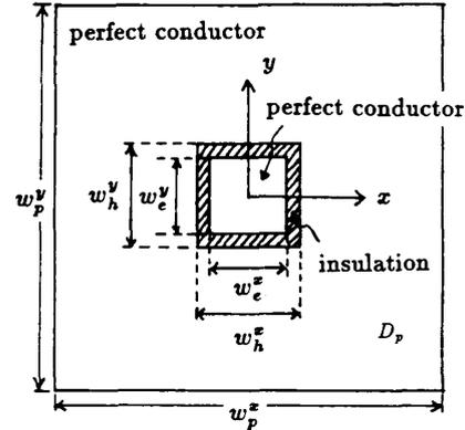
Fig. 2. Top view of the pad-electrode configuration.
