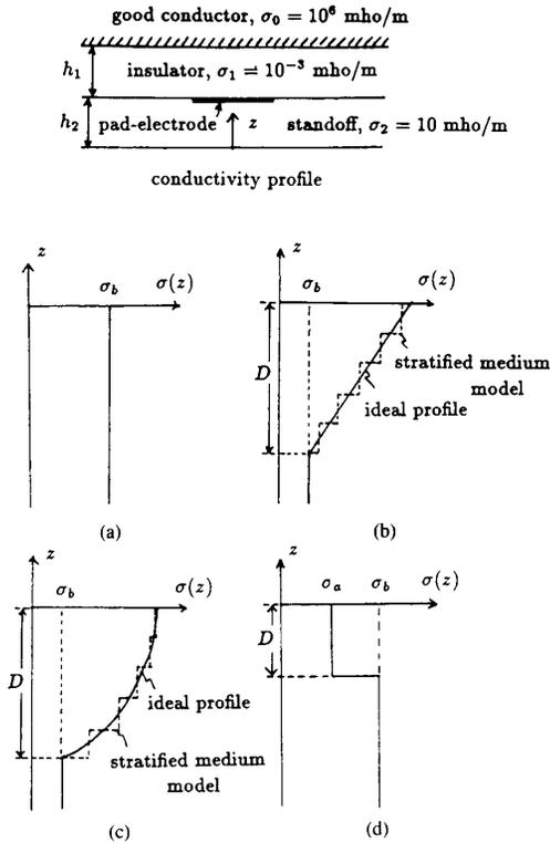
Fig. 8. Configuration of a pad-electrode in a profiled layered medium,  $w_p^x = w_p^y = 10$  cm,  $w_h^x = w_h^y = 2$  cm,  $w_e^x = w_e^y = 1.6$  cm,  $V_p = V_e = 1$  V. (a) Step profile. (b) Linear profile. (c) Parabolic profile. (d) Inversion profile.
