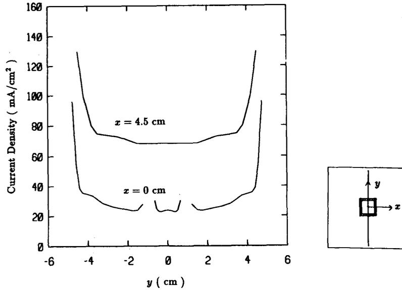
Fig. 3. Outflowing current distribution on a pad-electrode surface in a homogeneous medium with  $\sigma = 10$  S/m,  $w_p^x = w_p^y = 10$  cm,  $w_h^x = w_h^y = 2$  cm,  $w_e^x = w_e^y = 1.6$  cm,  $V_p = V_e = 1$  V.
