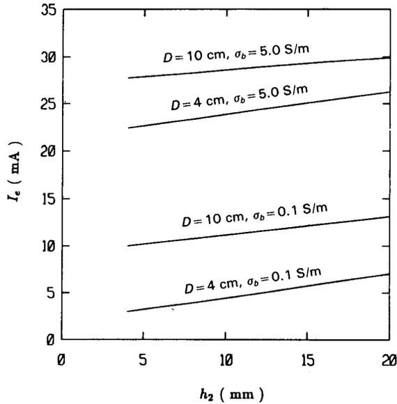
Fig. 11. Total electrode current of a pad-electrode with a linear conductivity profile,  $w_p^x = w_p^y = 10$  cm,  $w_h^x = w_h^y = 2$  cm,  $w_e^x = w_e^y = 1.6$  cm,  $V_p = V_e = 1$  V,  $h_1 = 2$  cm.
