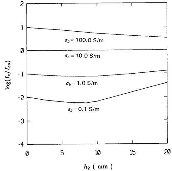
Fig. 9. Total electrode current of a pad-electrode with a step conductivity profile,  $w_p^x = w_p^y = 10$  cm,  $w_h^x = w_h^y = 2$  cm,  $w_e^x = w_e^y = 1.6$  cm,  $V_p = V_e = 1$  V,  $h_1 = 2$  cm,  $I_{e0}$  is the total electrode current when  $\sigma_b = 10$  S/m.
