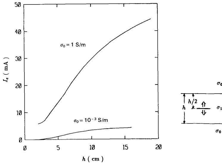
Fig. 5. Total electrode current of a pad-electrode in a three-layer medium,  $w_p^x = w_p^y = 10$  cm,  $w_h^x = w_h^y = 2$  cm,  $w_e^x = w_e^y = 1.6$  cm,  $V_p = V_e = 1$  V,  $\sigma_1 = 10$  S/m.
