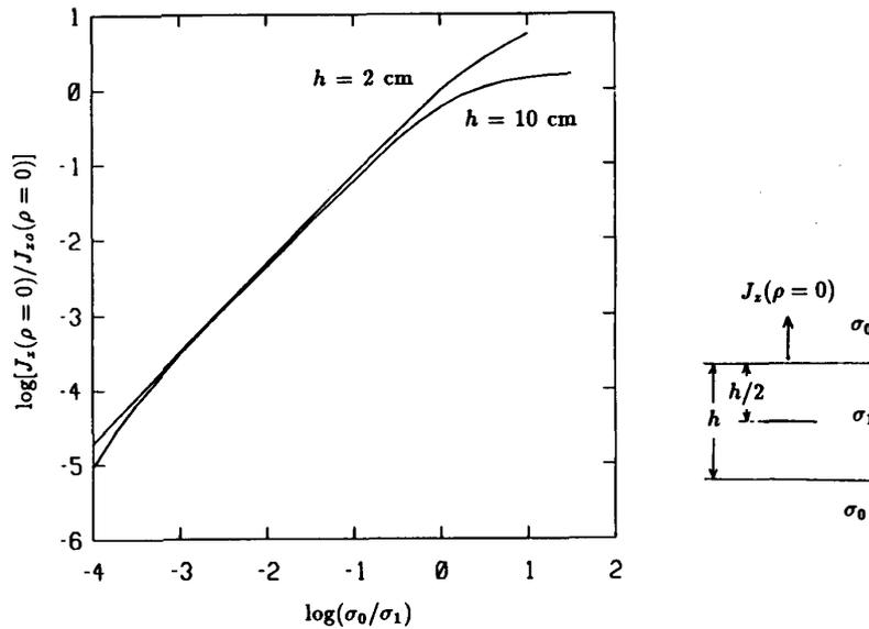
Fig. 6. Current density at the interface of a three-layer medium,  $w_p^x = w_p^y = 10$  cm,  $w_h^x = w_h^y = 2$  cm,  $w_e^x = w_e^y = 1.6$  cm,  $V_p = V_e = 1$  V,  $\sigma_1 = 10$  S/m,  $J_{z0}(\rho = 0)$  is the current density at 2 cm above the electrode with  $\sigma_0 = 10$  S/m.
