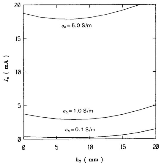
Fig. 10. Total electrode current of a pad-electrode with a step conductivity profile,  $w_p^x = w_p^y = 10$  cm,  $w_h^x = w_h^y = 2$  cm,  $w_e^x = w_e^y = 1.6$  cm,  $V_p = V_e = 1$  V,  $h_1 = 2$  cm.
