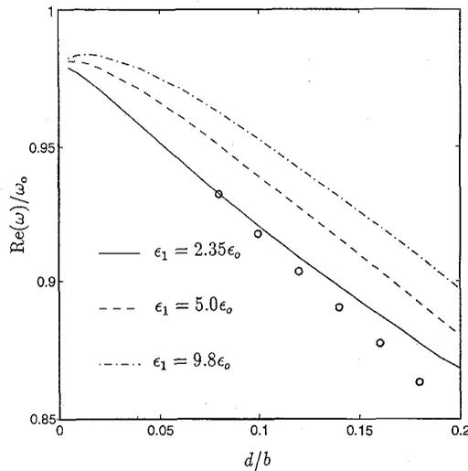
Fig. 2. Real part of (0, 1) mode resonance frequency of a rectangular patch resonator with one lamina of solid copper ground plane,  $a = 18$  cm,  $b = 10$  cm,  $\epsilon_0 = \epsilon_3 = \epsilon_o$ ,  $t_1 = 3$   $\mu\text{m}$ ,  $\epsilon'_{xx} = \epsilon'_{yy} = \epsilon'_{zz} = \epsilon_o$ ,  $\sigma'_{xx} = \sigma'_{yy} = \sigma'_{zz} = 5.8 \times 10^7$  U/m, o: results from [2].
