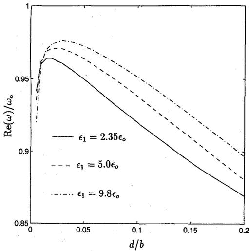
Fig. 4. Real part of (0, 1) mode resonance frequency of a rectangular patch resonator with a two-lamina G/E composite ground plane,  $a = 18$  cm,  $b = 10$  cm,  $\epsilon_0 = \epsilon_3 = \epsilon_o$ ,  $t_1 = t_2 = 25.4 \mu\text{m}$ ,  $\alpha_1 = 0$  degrees,  $\alpha_2 = 90$  degrees,  $\epsilon'_{xx} = \epsilon'_{yy} = \epsilon'_{zz} = 5.0\epsilon_o$ ,  $\sigma'_{xx} = 4 \times 10^4$  U/m,  $\sigma'_{yy} = \sigma'_{zz} = 50$  U/m.
