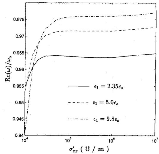
Fig. 6. Real part of (0, 1) mode resonance frequency of a rectangular patch resonator with a two-lamina G/E composite ground plane,  $a = 18$  cm,  $b = 10$  cm,  $\epsilon_0 = \epsilon_3 = \epsilon_o$ ,  $t_1 = t_2 = 25.4 \mu\text{m}$ ,  $\alpha_1 = 0$  degrees,  $\alpha_2 = 90$  degrees,  $\epsilon'_{xx} = \epsilon'_{yy} = \epsilon'_{zz} = 5.0\epsilon_o$ ,  $\sigma'_{yy} = \sigma'_{zz} = 50$  U/m.
