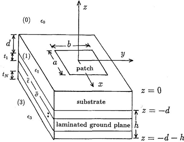
Fig. 1. A rectangular patch resonator in the presence of a laminated ground plane.
