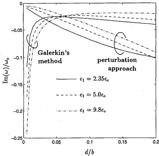
Fig. 5. Imaginary part of (0, 1) mode resonance frequency of a rectangular patch resonator with a two-lamina G/E composite ground plane. The parameters are the same as in Fig. 4.
