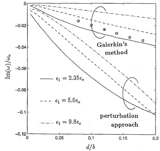
Fig. 3. Imaginary part of (0, 1) mode resonance frequency of a rectangular patch resonator with one lamina of solid copper ground plane. The parameters are the same as in Fig. 2.
