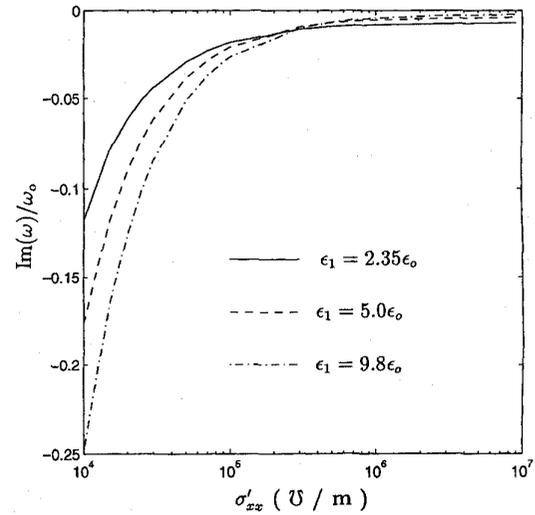
Fig. 7. Imaginary part of (0, 1) mode resonance frequency of a rectangular patch resonator with a two-lamina G/E composite ground plane. The parameters are the same as in Fig. 6.
