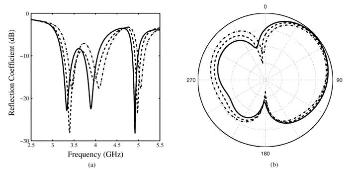
Fig. 7. Effect of two asymmetric wells on (a) reflection coefficient and (b) radiation patterns;  $\epsilon_r = 20$ ,  $a = 28$  mm,  $b = 9$  mm,  $d = 10$  mm,  $s_2 = s_4 = 7$  mm,  $s_1 = 2$  mm,  $L_s = 6$  mm,  $d_s = 7$  mm,  $L_a = 10$  mm,  $w_a = 2$  mm,  $W_g = L_g = 60$  mm, —:  $s_3 = 0.5$  mm, - - -:  $s_3 = 1$  mm, - · - ·:  $s_3 = 2$  mm.
