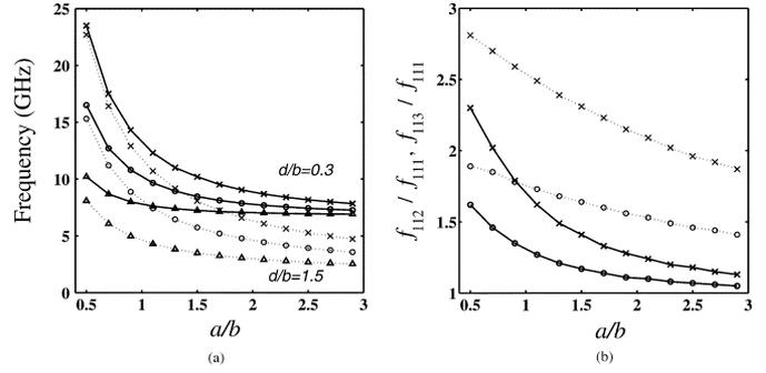
Fig. 2. (a) Resonant frequencies at different  $d/b$  ratios given  $a/b$  ratio. (b) Ratios of resonant frequencies of  $TE_{112}^y$  and  $TE_{113}^y$  modes with respect to that of  $TE_{111}^y$  mode. —:  $d/b = 0.3$ ; ...:  $d/b = 1.5$ ,  $\Delta$ :  $TE_{111}^y$  mode;  $\circ$ :  $TE_{112}^y$  mode;  $\times$ :  $TE_{113}^y$  mode;  $\epsilon_r = 20$ ;  $b = 9$  mm.
