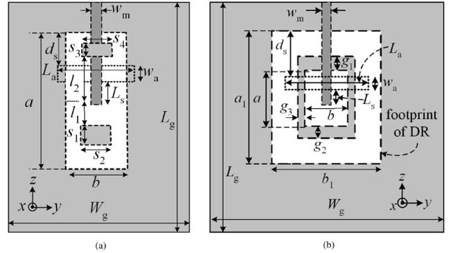
Fig. 6. (a) Configuration of DR antenna embedded with two asymmetric wells. (b) DR antenna with a moat and feed network.
