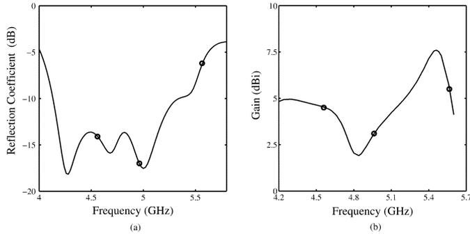
Fig. 8. (a) Simulated reflection coefficient and (b) gain of  $E_\theta$  pattern at  $\theta = 90^\circ$ ,  $\epsilon_r = 20$ ,  $a = 30$  mm,  $b = 19$  mm,  $d = 4$  mm,  $d_s = 12$  mm,  $w_a = 1$  mm,  $L_a = 7$  mm,  $L_s = 4$  mm,  $W_g = L_g = 70$  mm;  $\circ$  marks the resonant frequencies of  $\text{TE}_{111}^y$ ,  $\text{TE}_{112}^y$ , and  $\text{TE}_{113}^y$  modes, respectively.
