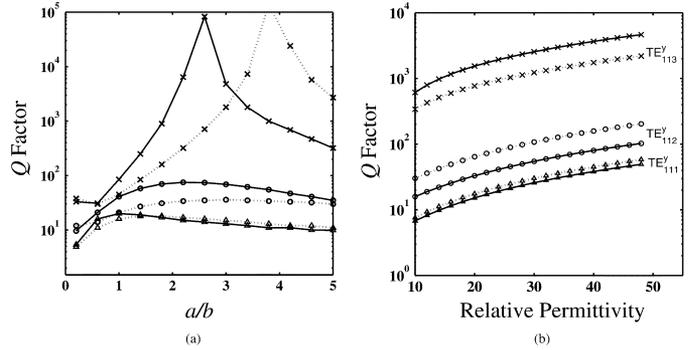
Fig. 3. (a)  $Q$  factors at different  $d/b$  ratios given  $a/b$  ratio. —:  $d/b = 0.5$ ; ...:  $d/b = 1$ ; ...:  $d/b = 1.89$ ;  $\epsilon_r = 20$ ;  $b = 9$  mm. (b)  $Q$  factors at different permittivities.  $b = 9$  mm; —:  $a/b = 3.1$ ;  $d/b = 1.1$ ; ...:  $a/b = 1.89$ ;  $d/b = 0.56$ ;  $\Delta$ :  $TE_{111}^y$ ;  $\circ$ :  $TE_{112}^y$ ;  $\times$ :  $TE_{113}^y$ .
