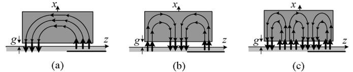
Fig. 4. Electric field distribution within gap and DR: (a)  $TE_{111}^y$  mode, (b)  $TE_{112}^y$  mode, (c)  $TE_{113}^y$  mode.
