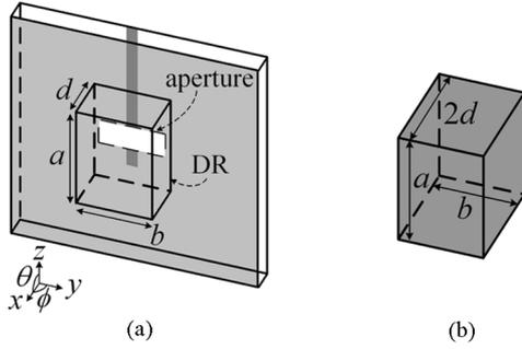
Fig. 1. (a) DR on a ground plane. (b) Equivalent DR in free space.
