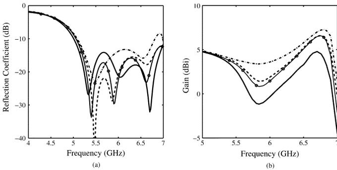
Fig. 9. Effect of  $d_s$  on (a) reflection coefficient and (b) gain at  $\theta = 90^\circ$  and  $\phi = 0^\circ$ ,  $-\cdot-$ :  $d_s = 12$  mm,  $-\cdot-\cdot-$ :  $d_s = 13$  mm,  $-\cdot-\cdot-\cdot-$ :  $d_s = 14$  mm,  $-\circ-\cdot-$ :  $d_s = 16$  mm,  $\epsilon_r = 20$ ,  $a = 17$  mm,  $b = 10$  mm,  $a_1 = 30.5$  mm,  $b_1 = 19$  mm,  $d = 4$  mm,  $g_1 = g_2 = 2.75$  mm,  $g_3 = 0.5$  mm,  $L_s = 4$  mm,  $L_a = 12$  mm,  $w_a = 2$  mm,  $W_g = L_g = 70$  mm.
