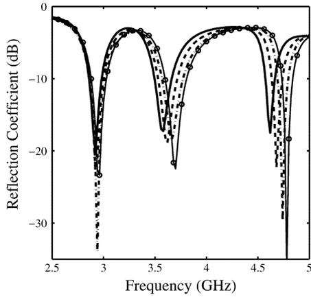
Fig. 5. Effect of gap between DR and ground plane;  $\epsilon_r = 20$ ,  $a = 28$  mm,  $b = 9$  mm,  $d = 10$  mm,  $L_s = 6$  mm,  $d_s = 7$  mm,  $L_a = 10$  mm,  $w_a = 2$  mm,  $W_g = L_g = 60$  mm, —:  $g = 0$  mm, - - -:  $g = 0.01$  mm, - · - ·:  $g = 0.02$  mm, · · ·:  $g = 0.03$  mm.
