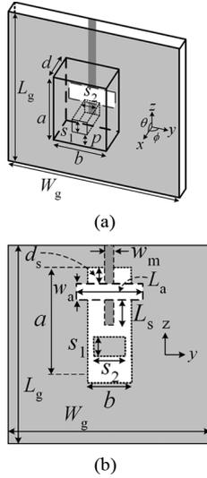
Fig. 1. (a) Configuration of DR antenna with a well. (b) Top view.
