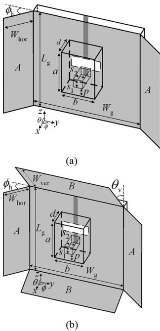
Fig. 2. DR antenna with a well on a finite ground plane. (a) Two plates with mark A are attached to vertical edges of ground plane. (b) Two plates with mark B are attached to horizontal edges of ground plane.
