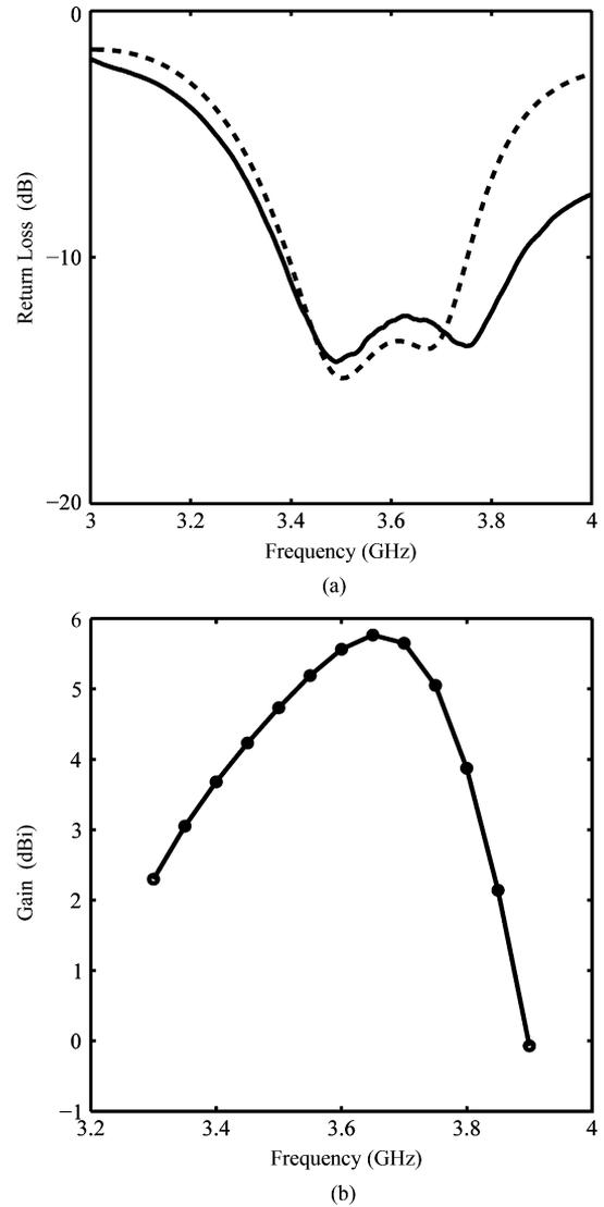
Fig. 7. Return loss of DR antenna with broadside radiation pattern,  $a = 21$  mm,  $b = 13.5$  mm,  $d = 9.7$  mm,  $s_1 = 5.4$  mm,  $s_2 = 9.1$  mm,  $p = 8.5$  mm,  $w_a = 1$  mm,  $L_a = 12.5$  mm,  $d_s = 2.6$  mm,  $l_s = 3$  mm,  $W_{ver} = W_{hor} = 60$  mm,  $\phi_h = 85^\circ$ ,  $\theta_v = 75^\circ$ ,  $\epsilon_r = 20$ ,  $W_x = 80$  mm,  $W_y = 55$  mm,  $\bullet$ : measurement,  $-\cdot-\cdot-$ : simulation. (b) Antenna gain at ( $\theta = 90^\circ$ ,  $\phi = 0^\circ$ ).
