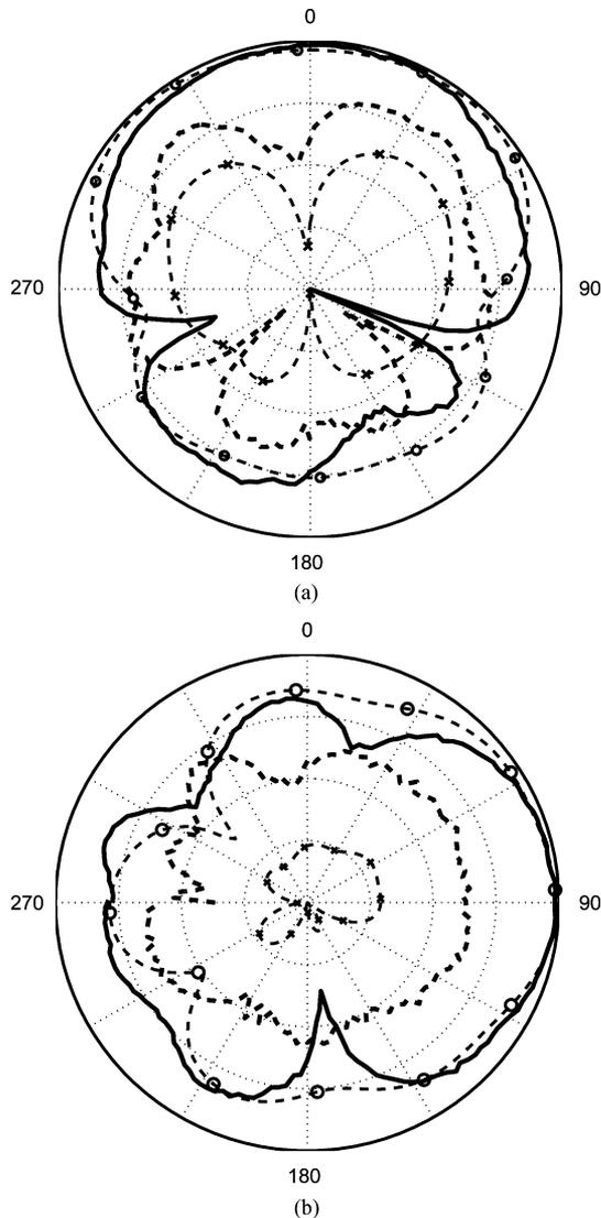
Fig. 8. Measured radiation patterns of the DR antenna in (a)  $xy$ -plane. (b)  $xz$ -plane, all parameters are the same as in Fig. 7, 10 dB per division on the radial,  $-$ : measured  $E_\theta$ ,  $- - -$ : measured  $E_\phi$ ,  $- \circ -$ : simulated  $E_\theta$ ,  $- \times -$ : simulated  $E_\phi$ .
