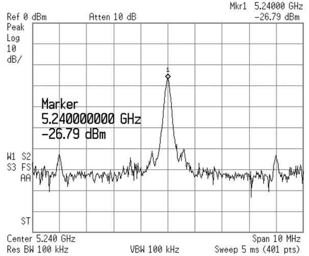
Fig. 15. Measured output spectrum of the synthesizer.
