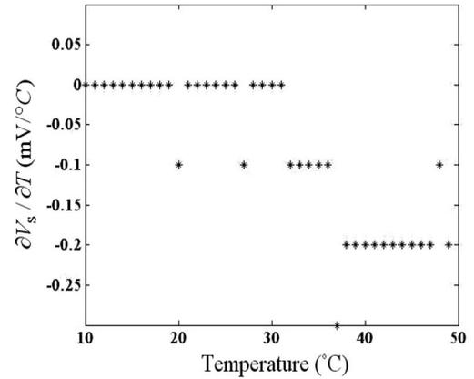
Fig. 6. TC at  $V_S$ , with  $V_o = 1.316$  V.
