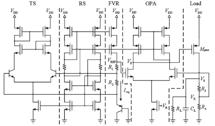
Fig. 4. Schematic of proposed regulator: TS: temperature stabilizer; RS: ripple stabilizer; FVR: fixed voltage reference; OPA: operational amplifier.
