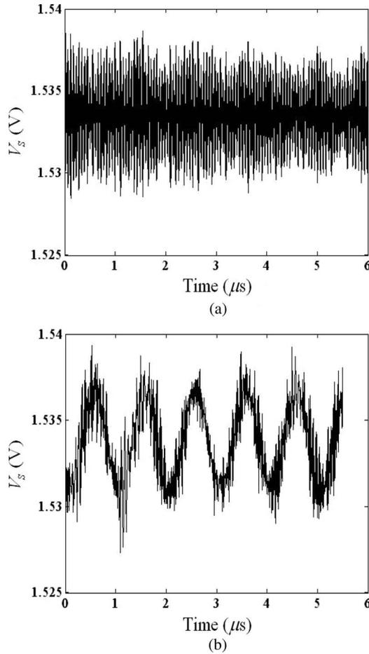
Fig. 5. Variation of  $V_S$  with a perturbation of  $A_r \times \sin(2\pi \times 10^6 t)$  mV superimposed on  $V_{DD}$ . (a)  $A_r = 50$  mV. (b)  $A_r = 200$  mV.
