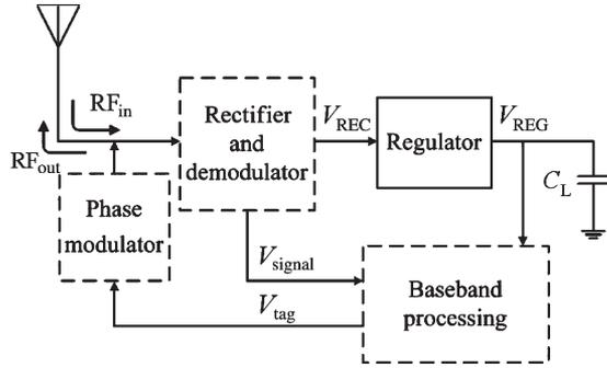
Fig. 1. Voltage regulator for RFID tag.
