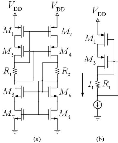
Fig. 2. Schematic of the ripple stabilizer. (a) Cascode current mirror. (b) Diodelike pair with self-bias.
