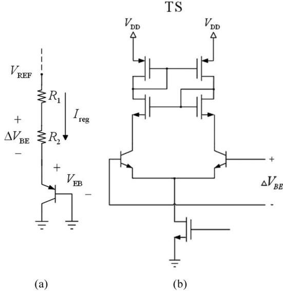
Fig. 3. Schematic of bandgap reference generator. (a) Zero-TC voltage reference. (b)  $\Delta V_{BE}$  generation circuit, TS stands for temperature stabilizer.
