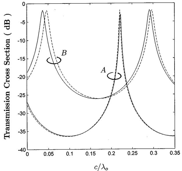
Fig. 4. Transmission cross section of a bent slot in a plate,  $\theta_i = 0$ ,  $\epsilon_i = \epsilon_o$  with  $0 \leq i \leq 6$ , —: bent slot, ---: straight slot with the same length and width as the bent slot. A: plate thickness is  $0.03\lambda_o$ , slot width is  $0.003\lambda_o$ ,  $b = 0.003\lambda_o$ , B: plate thickness is  $0.3\lambda_o$ , slot width is  $0.01\lambda_o$ ,  $b = 0.03\lambda_o$ .
