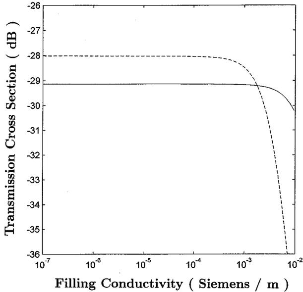
Fig. 6. Effect of filling conductivity on the transmission cross section of a bent slot in a plate  $0.03\lambda_o$  thick, slot width is  $0.003\lambda_o$ ,  $b = 0.006\lambda_o$ ,  $\theta_i = 0^\circ$ ,  $\epsilon_i = \epsilon_o$  and  $\sigma_i = \sigma$  with  $1 \leq i \leq 5$ ,  $\epsilon_i = \epsilon_o$  and  $\sigma_i = 0$  with  $i = 0$  and  $6$ , —:  $c = 0.006\lambda_o$ , - - -:  $c = 0.25\lambda_o$ .
