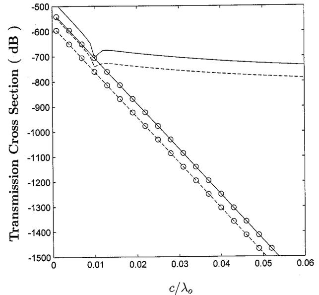
Fig. 8. Transmission cross section of a bent slot in a plate  $0.03\lambda_o$  thick, slot width is  $0.003\lambda_o$ ,  $\theta_i = 0$ ,  $\epsilon_i = \epsilon_o$  with  $0 \leq i \leq 6$ , —: bent slot with  $b = 0.003\lambda_o$ , —o—: straight slot with the same length as the bent slot ( $b = 0.003\lambda_o$ ), - - -: bent slot with  $b = 0.006\lambda_o$ , - - -o- -: straight slot with the same length as the bent slot ( $b = 0.006\lambda_o$ ).
