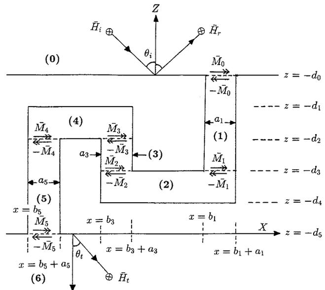
Fig. 1. Configuration of a bent slot exposed to an incident TM plane wave.
