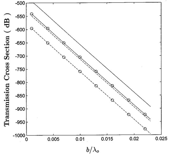
Fig. 7. Transmission cross section of a bent slot in a plate  $0.03\lambda_o$  thick, slot width is  $0.003\lambda_o$ ,  $\theta_i = 0$ ,  $\epsilon_i = \epsilon_o$  with  $0 \leq i \leq 6$ , —: bent slot with  $c = 0.003\lambda_o$ , —o—: straight slot with the same length as the bent slot ( $c = 0.003\lambda_o$ ), - - -: bent slot with  $c = 0.006\lambda_o$ , - - -o- -: straight slot with the same length as the bent slot ( $c = 0.006\lambda_o$ ).
