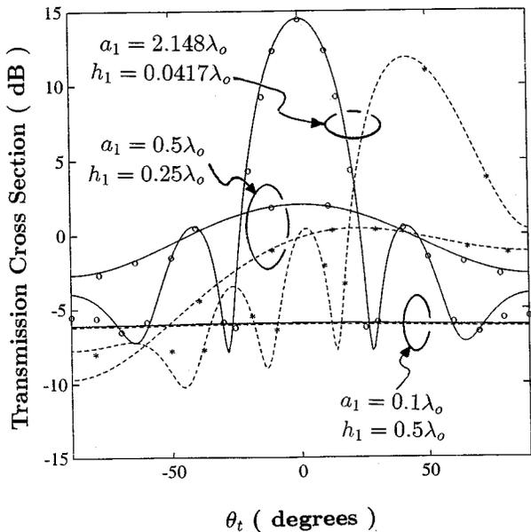
Fig. 2. Transmission cross section of a straight slot in a thick plate. —:  $\theta_i = 0^\circ$ , ---:  $\theta_i = 45^\circ$ , o: results in [5] ( $\theta_i = 0^\circ$ ), \*: results in [5] ( $\theta_i = 45^\circ$ ).
