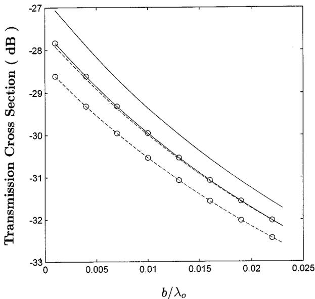
Fig. 3. Transmission cross section of a bent slot in a plate  $0.03\lambda_o$  thick, slot width is  $0.003\lambda_o$ ,  $\theta_i = 0$ ,  $\epsilon_i = \epsilon_o$  with  $0 \leq i \leq 6$ , —: bent slot with  $c = 0.003\lambda_o$ , ---: straight slot with the same length as the bent slot ( $c = 0.003\lambda_o$ ), -.-: bent slot with  $c = 0.006\lambda_o$ , .-.: straight slot with the same length as the bent slot ( $c = 0.006\lambda_o$ ).
