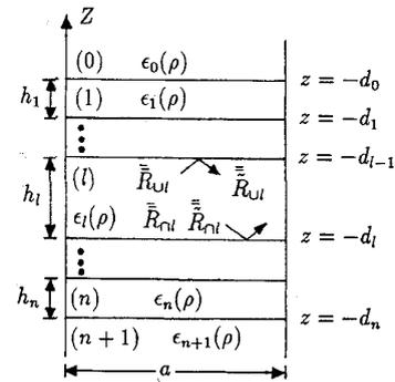
Fig. 1. Geometrical configuration of cascaded circular waveguide sections loaded with inhomogeneous dielectrics.
