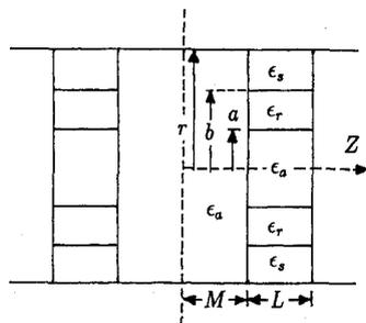
Fig. 2. Resonant frequencies of the TE<sub>01δ</sub> mode of two symmetrically coupled dielectric ring resonator,  $\epsilon_r(\rho) = 24.3 + 4(\epsilon_m - 24.3)(\rho - a)(b - \rho)/(b - a)^2$ ,  $\epsilon_s = 1.031$ ,  $\epsilon_a = 1$ ,  $b = 2.455$  mm,  $a = 0.3b$ ,  $r = 2.39b$ ,  $(b/L)^2 = 0.4625$ . —: electric wall in the middle. - - - -: magnetic wall in the middle (results from [3]).
