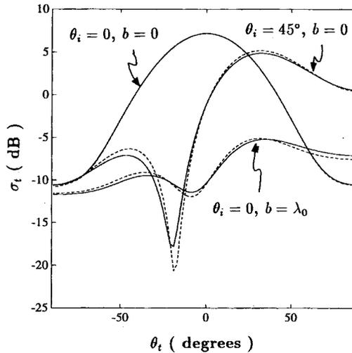
Fig. 4. Transmission cross section through slits on stacked thick plates.  $a = \lambda_0$ ,  $h_1 = 0.001\lambda_0$ ,  $h_2 = 0.25\lambda_0$ ,  $h_3 = 0.001\lambda_0$ ,  $\epsilon_1 = \epsilon_2 = \epsilon_3 = \epsilon_o$ , —: finite thickness approach, - - - : zero-thickness approach.
