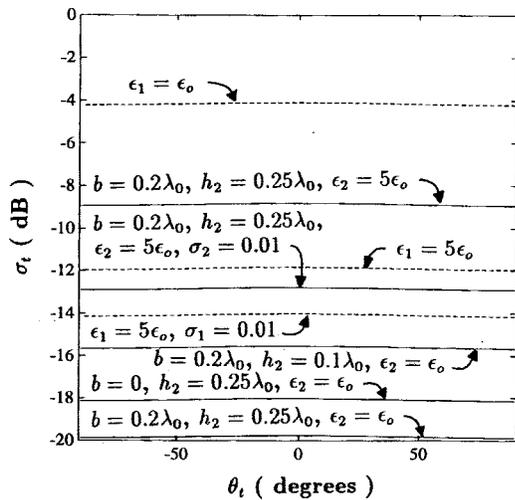
Fig. 5. Transmission cross section through slits on single and stacked thick plates.  $\theta_i = 0$ ,  $a = 0.1\lambda_0$ , for single plate:  $h_1 = 0.5\lambda_0$ , for stacked plates:  $h_1 = h_3 = 0.25\lambda_0$ ,  $\epsilon_1 = \epsilon_3 = \epsilon_0$ , —: stacked plates, - - -: single plate.
