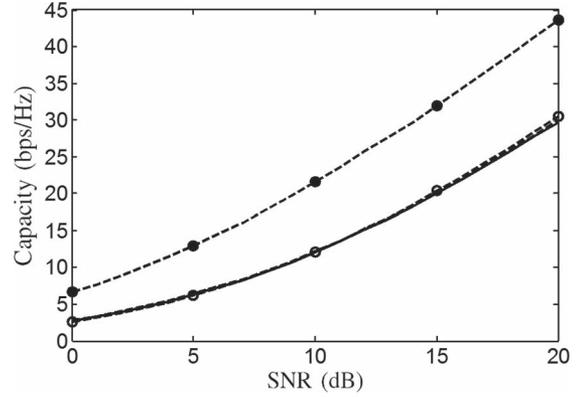
Fig. 5. Capacity of an  $8 \times 8$  MIMO system over a channel with single-cluster Laplacian PAS,  $\phi_0 = 90^\circ$ ,  $\phi_1 = 90^\circ$ ,  $\sigma_L = 45^\circ$ , and  $\Delta\phi = 90^\circ$ ; 1000 Monte Carlo channel realizations at each SNR. (a) Strategy of uniformly distributed transmitting power: —: using (16); - - -: using  $\bar{H}'_c$  in (13); - o -: using  $\bar{H}_c$  in (7); and - • -: using  $\bar{H}$  in (4).
