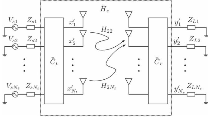
Fig. 1.  $N_t \times N_r$  MIMO channel, with mutual coupling among antennas in the same array.
