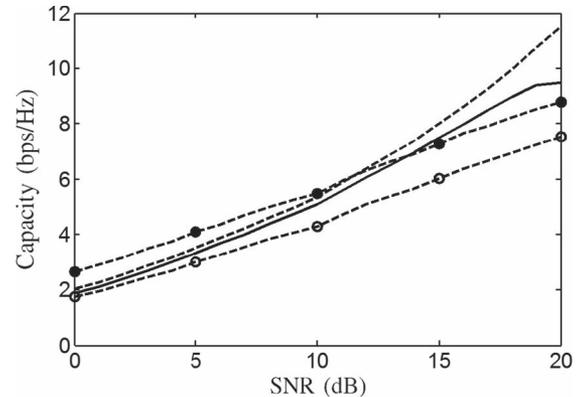
Fig. 3. Capacity of an  $8 \times 8$  MIMO system over an LOS channel with the same parameters as in Fig. 2, except  $\phi_0 = 90^\circ$ . Strategy of uniformly distributed transmitting power: —: using (16); - - -: using  $\bar{H}'_c$  in (13); - o -: using  $\bar{H}_c$  in (7); - • -: using  $\bar{H}$  in (4).
