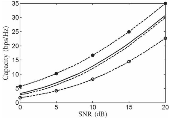
Fig. 4. Capacity of an  $8 \times 8$  MIMO system over a channel with single-cluster Laplacian PAS,  $\phi_0 = 90^\circ$ ,  $\phi_1 = 15^\circ$ ,  $\sigma_L = 30^\circ$ , and  $\Delta\phi = 60^\circ$ ; 1000 Monte Carlo channel realizations at each SNR. Strategy of uniformly distributed transmitting power: —: using (16); - - -: using  $\bar{H}'_c$  in (13); - o -: using  $\bar{H}_c$  in (7); - • -: using  $\bar{H}$  in (4).
