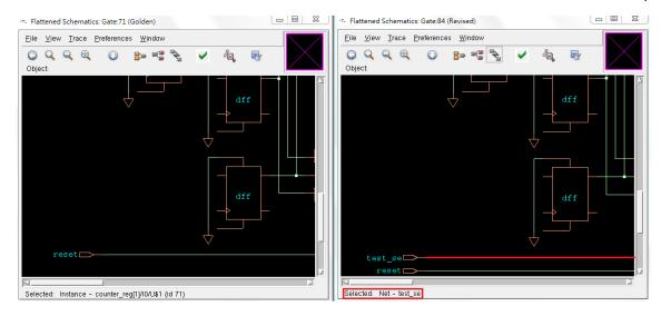
From schematic views of corresponding DFF, we can found that in the revised schematic, an extra input *test\_se* is found at the input cone of that DFF. Recall that this input is added for test mode toggling in DFT design, with fixed value 1 for scan mode instead of function mode of the design. What happened once LEC set this input to be 1?! Will the two DFF report the same result?! Will they be proved equivalent?! Why?!
