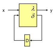
**Given:** Finite-State Machine  $F(Q,X,Y,\delta,\lambda)$  where:
