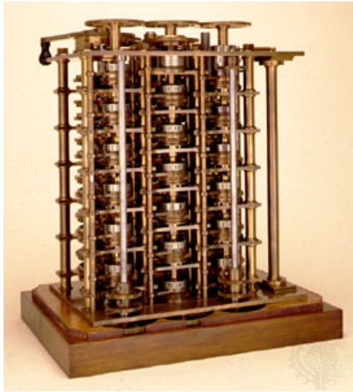
Babbage's difference engine (1822) powered by cranking a handle
