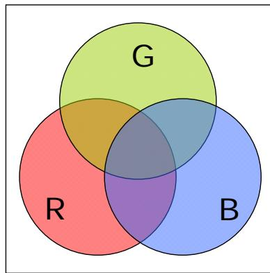
$$(R \cap G) \cup (R' \cap B) \cup (G \cap B) = (R \cap G) \cup (R' \cap B)$$
