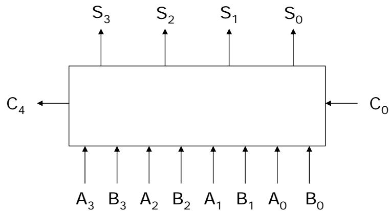
Method 1: Design from constructing a truth table of the whole system (**difficult simplification and complex implementation**)
