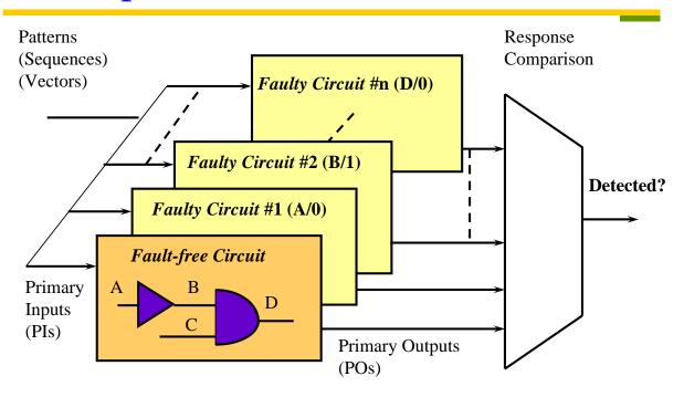
Logic simulation on both good (fault-free) and faulty circuits
