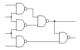
\* 30 total faults  $\rightarrow$  12 prime faults
