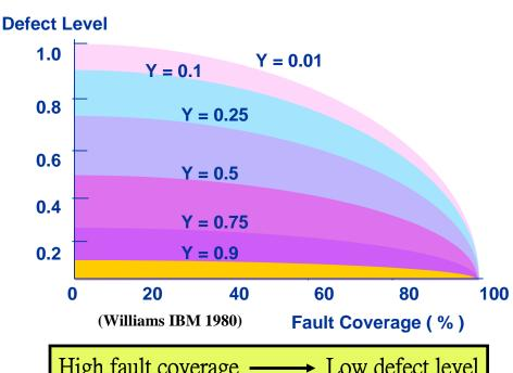
High fault coverage — Low defect level
