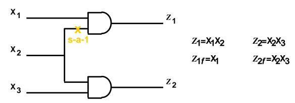
Test  $(x_{1},x_{2},x_{3}) = (100)$  detects f because  $z_{1}(100)=0$  and  $z_{1f}(100)=1$
