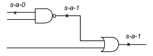
Three faults shown are equivalent!
