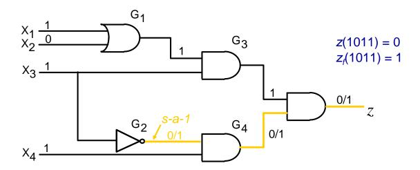
Input vector 1011 detects the fault f ( $G_2$  stuck-at-1)  $v/v_f$ : v = signal value in the fault free circuit
