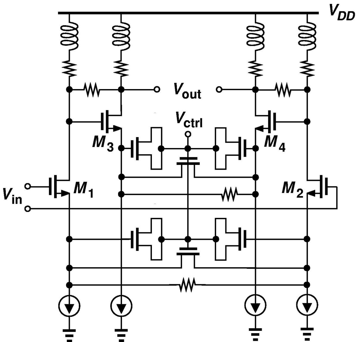
Figure 4.7.3: Equalizing filter stage.
