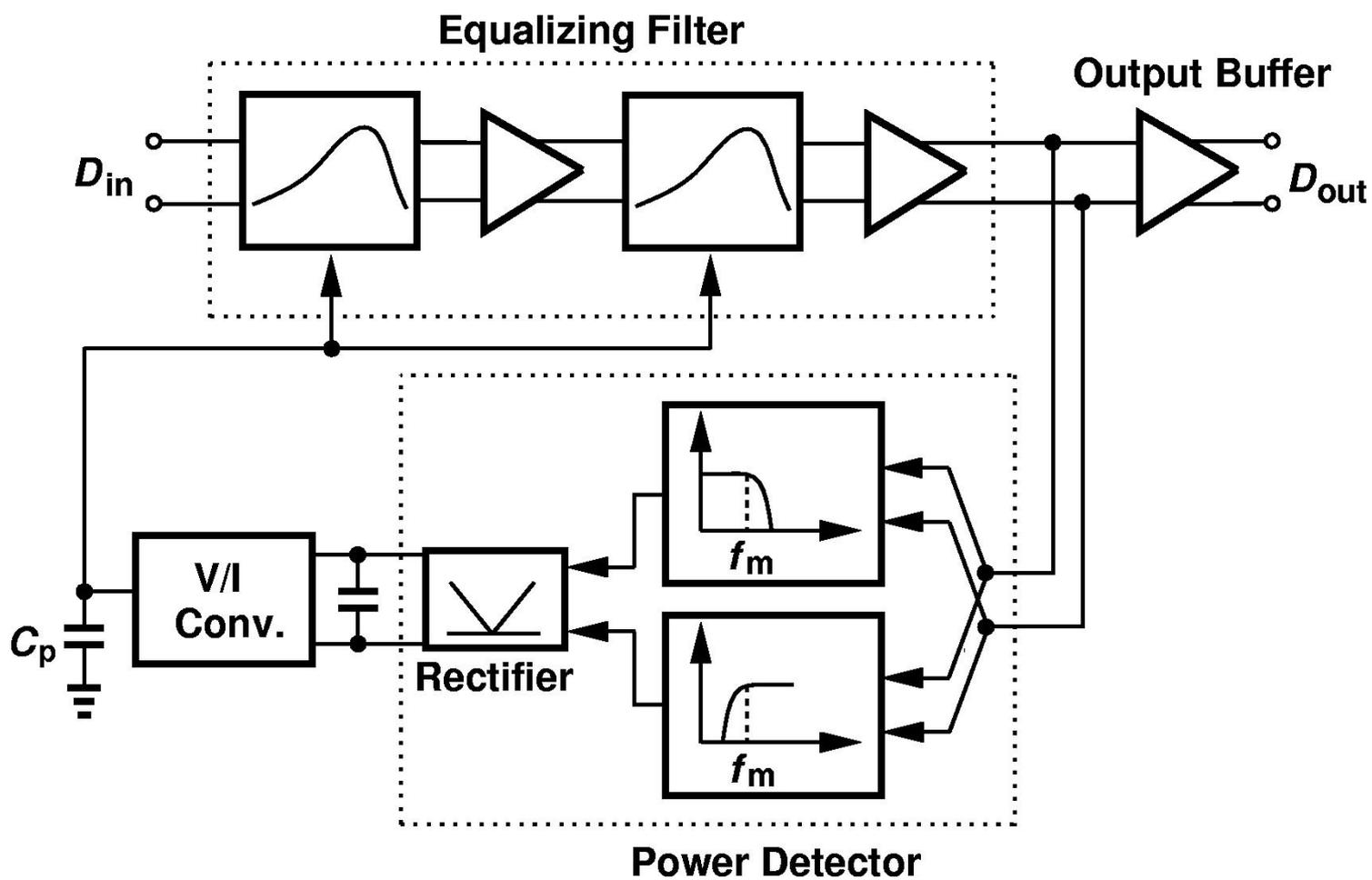
Figure 4.7.2: Equalizer architecture.
