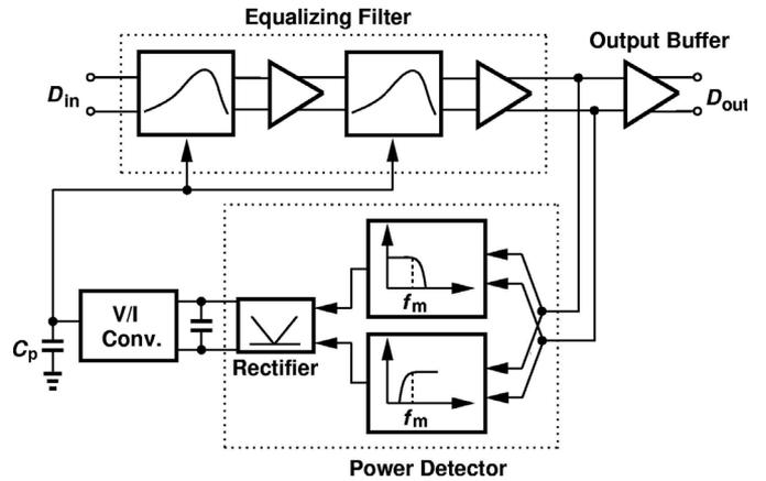
Figure 4.7.2: Equalizer architecture.
