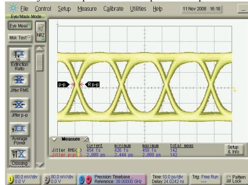
Fig. 7. Transmitter output at 39 Gb/s.
