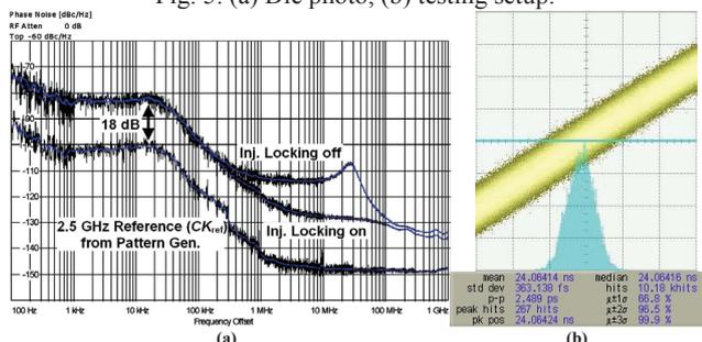
Fig. 6. (a) Phase noise, (b) time-domain jitter (vertical scale: 10 mV/div, horizontal scale: 1 ps/div) of the CMU output ( $CK_{20G}$ ).
