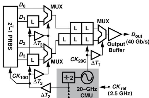
Fig. 1. Transmitter architecture.
