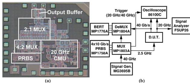
Fig. 5. (a) Die photo, (b) testing setup.
