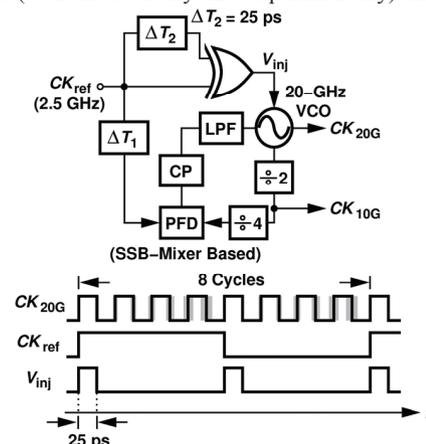
Fig. 3. CMU design with subharmonic injection locking.
