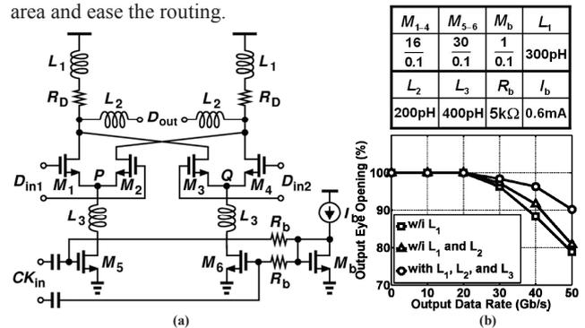
Fig. 2. (a) 40-Gb/s selector designs, (b) eye opening comparison.
