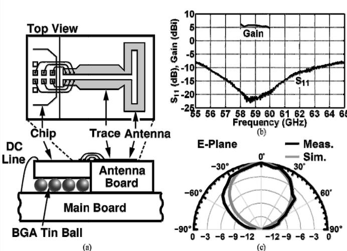
Figure 18.6.5: (a) Chip and antenna assembly, (b)  $S_{11}$  and gain of the dipole antenna (equipment limited), (c) antenna pattern (E-plane).
