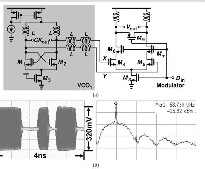
Figure 18.6.2: (a) VCO1 and OOK modulator, (b) measured OOK signals at PA output (left: 2.5Gb/s, right: 1Gb/s).
