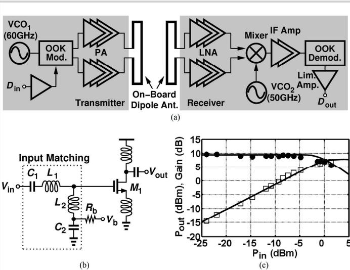
Figure 18.6.1: (a) Transceiver architecture, (b) one PA stage, (c) measured gain and  $P_{out}$  of PA.
