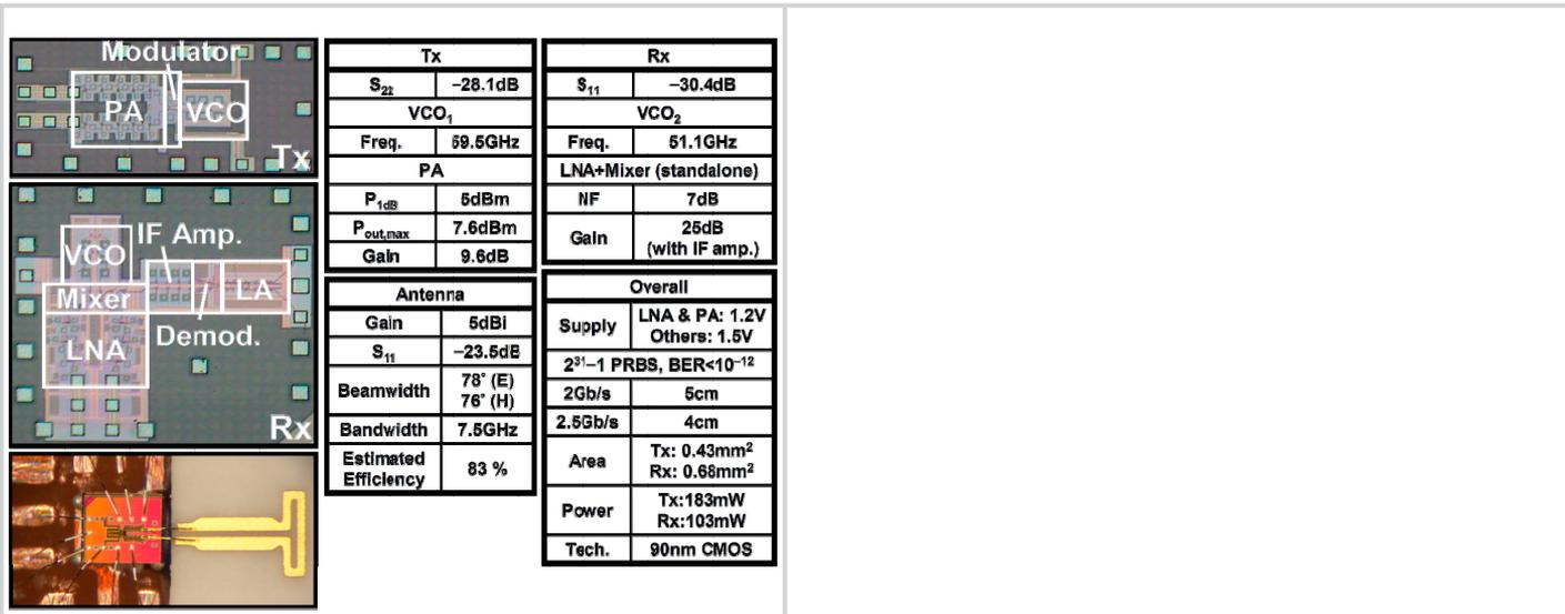
Figure 18.6.7: Die micrograph, testing board, and performance summary.
