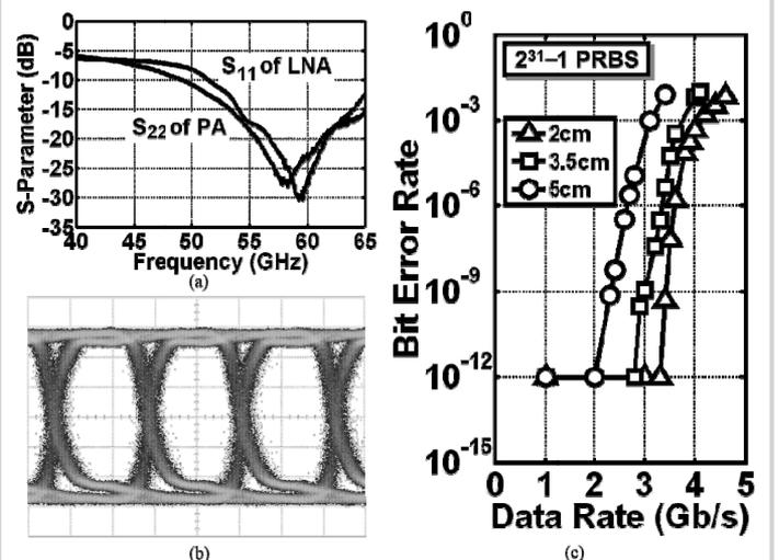
Figure 18.6.6: (a) Input/Output matching of the transceiver, (b) recovered data at 3Gb/s (vertical scale: 60mV/div, horizontal scale: 150ps/div), (c) BER test.
