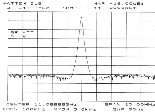
Fig. 18. Recovered clock spectrum of the 10-Gb/s prototype.
