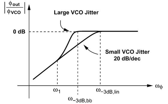
Fig. 12. Transfer function of VCO phase noise.
