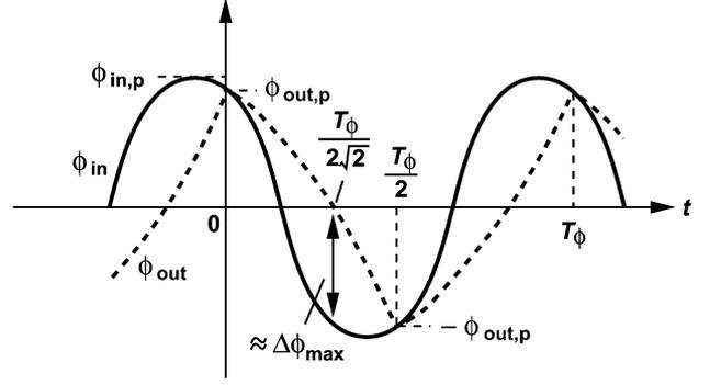
Fig. 10. Nonlinear slewing in jitter tolerance test.
