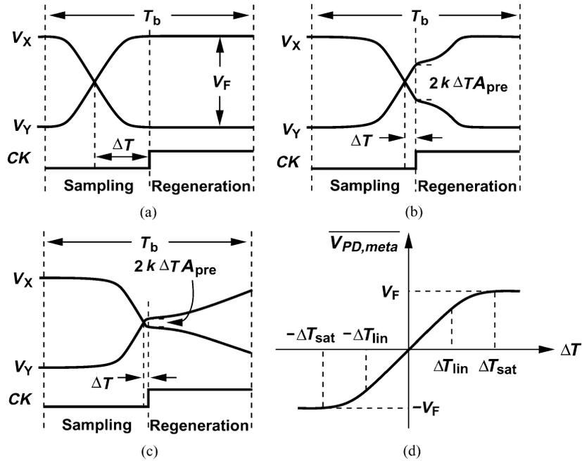
Fig. 2. (a) Average PD output for complete differential pair switching. (b) Average PD output for partial differential pair switching but full regeneration. (c) Average PD output for incomplete regeneration. (d) Typical bang-bang characteristic.
