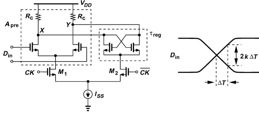
Fig. 1. Current-steering latch and its input data waveform.
