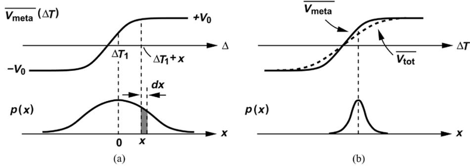
Fig. 5. (a) Derivation of overall characteristic. (b) Result for small jitter.
