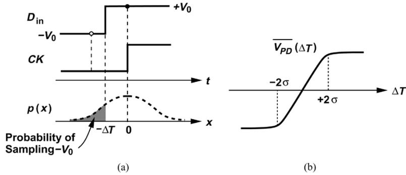
Fig. 4. Smoothing of PD characteristic due to jitter.
