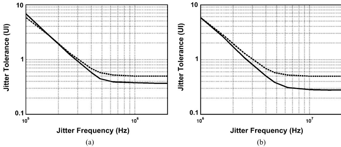
Fig. 16. Measured (solid lines) and predicted (dashed lines) jitter tolerance of (a) 1-Gb/s prototype and (b) 10-Gb/s prototype.
