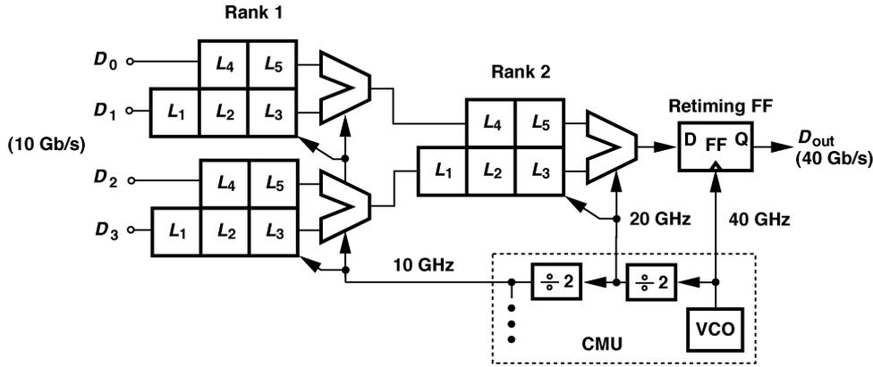
Fig. 1. Conventional realization of a 40-Gb/s transmitter with 4:1 MUX.
