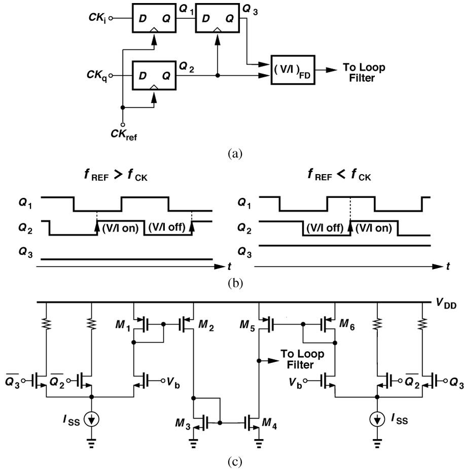
Fig. 11. (a) Frequency detector; (b) its operation; (c) realization of  $(V/I)_{FD}$ .
