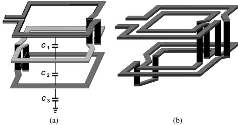
Fig. 7. Differentially stacked inductors with multiple layers and turns. (a) Three layers. (b) Multiple turns and layers.
