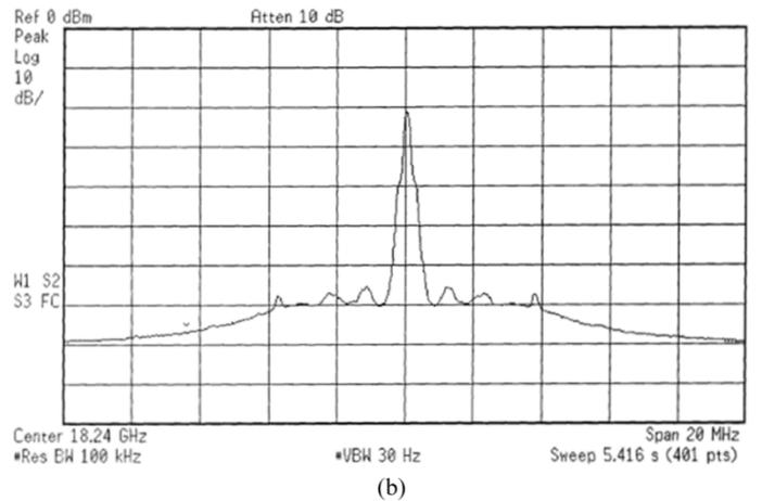
Fig. 20. (a) Clock jitter measurement (horizontal scale: 2 ps/div, vertical scale: 10 mV/div). (b) Output spectrum under locked condition.
