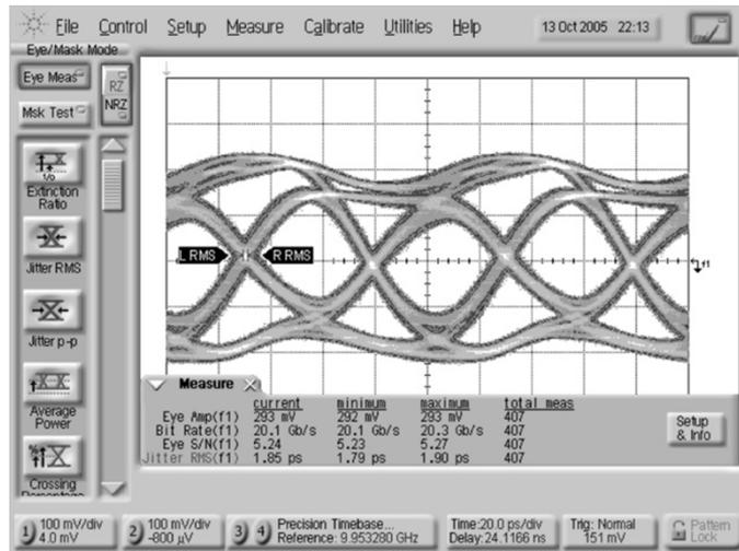
Fig. 15. Output waveform of the MUX operating at 20 Gb/s.
