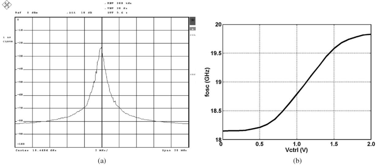
Fig. 19. (a) Free-running spectrum (center: 18.47 GHz, span: 20 MHz, RBW: 300 kHz). (b) Tuning range of the VCO in the CMU circuit.
