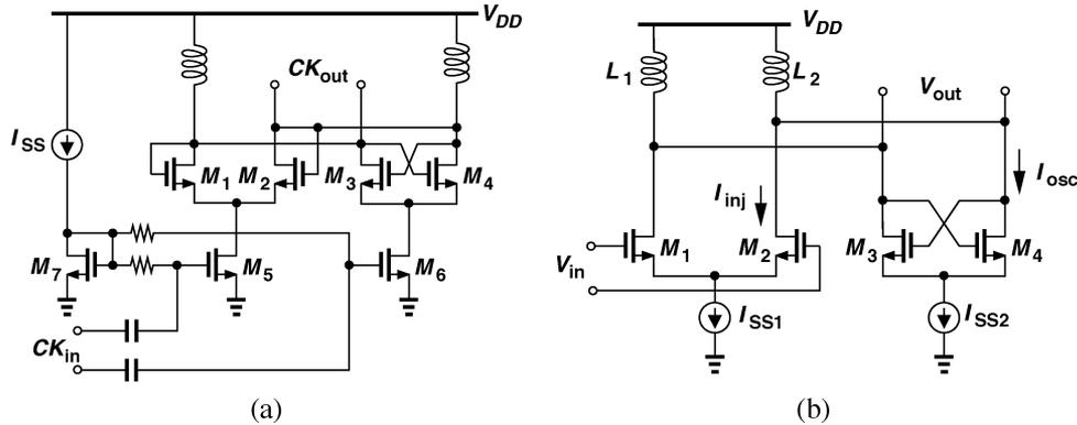
Fig. 12. (a) First  $\div 2$  circuit. (b) Clock buffer.
