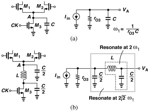
Fig. 2. Internal node behavior (a) without and (b) with series inductor.
