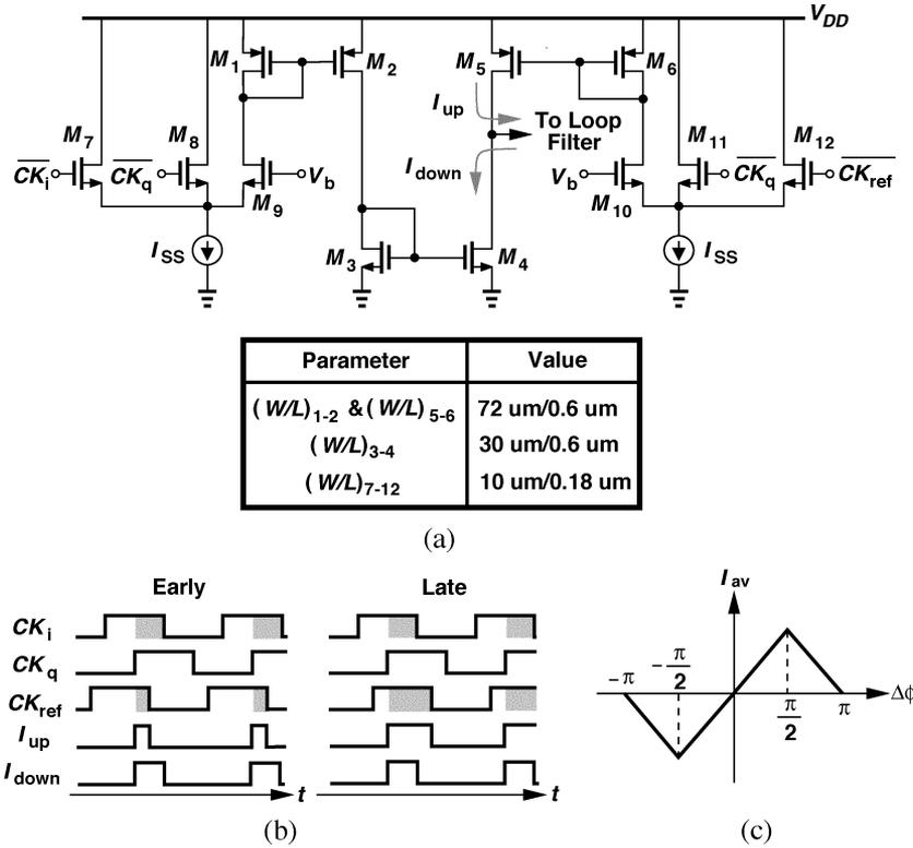
Fig. 10. (a) Phase detector and  $V$ -to- $I$  converter; (b) timing diagram; (c) its characteristic.TABLE II
