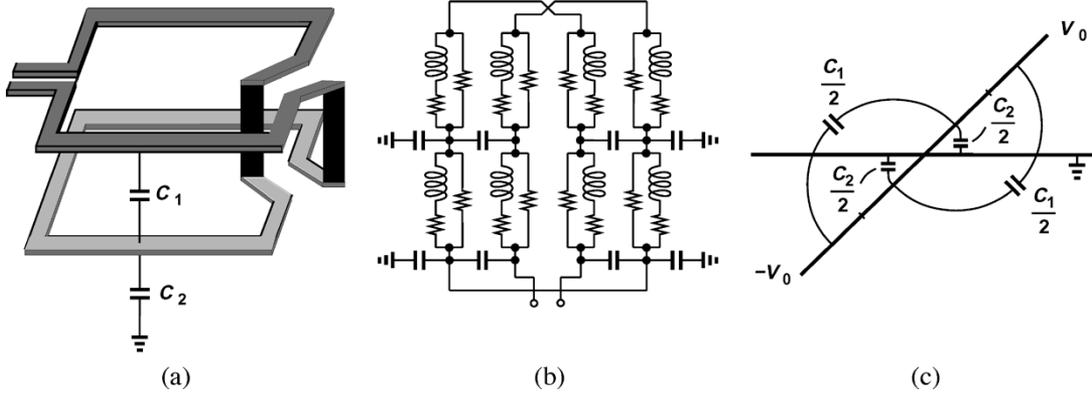
Fig. 6. (a) Proposed differentially stacked inductor; (b) its model; (c) the voltage profile.
