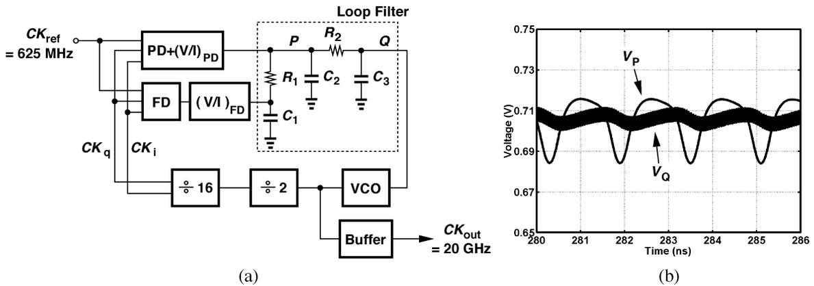
Fig. 9. (a) CMU architecture. (b) Simulated waveforms of \$V\_P\$ and \$V\_Q\$.
