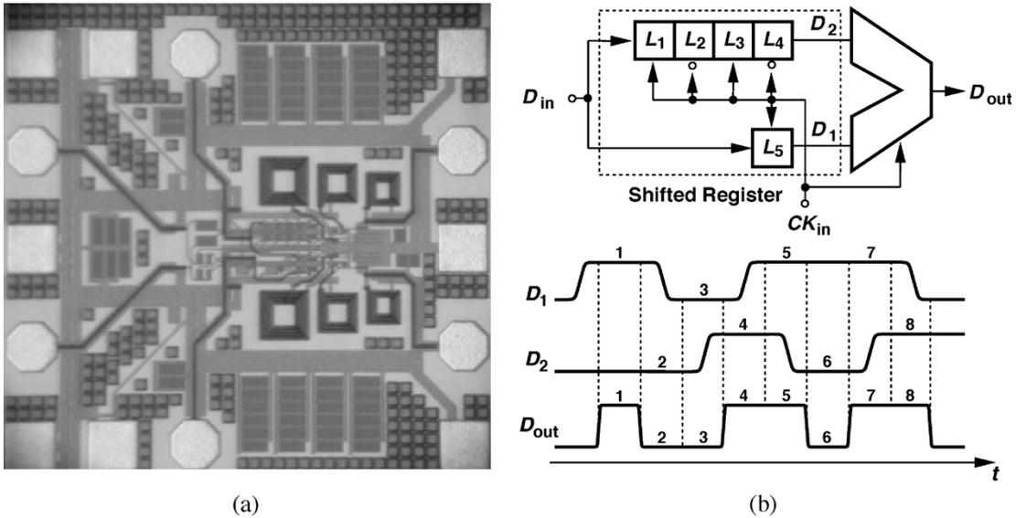
Fig. 14. (a) Chip photo of MUX. (b) Generation of input data.
