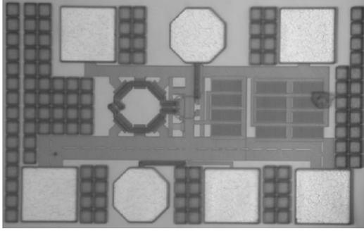
Fig. 16. Chip micrograph of VCO and the testing setup.
