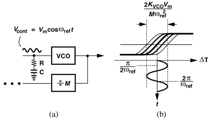
Fig. 13. Jitter due to control-line ripple.
