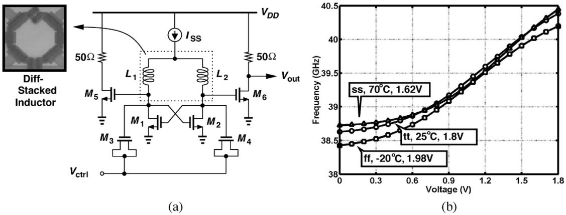
Fig. 8. (a) VCO design and its parameters. (b) Tuning curves under process, temperature, and supply variations.
