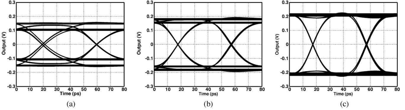
Fig. 5. Output data for: (a) conventional current-steering selector; (b) current-steering selector with inductive peaking; (c) proposed selector.
