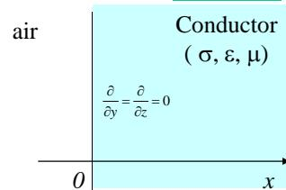
$$\nabla \times \nabla \times \vec{E} = -j\omega\mu\nabla \times \vec{H} = -j\omega\mu\sigma\vec{E};$$
