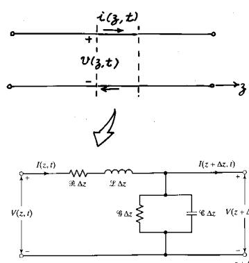
$$\left\{ \begin{array}{l} -\frac{\partial v}{\partial z} = R \cdot i + L \cdot \frac{\partial i}{\partial t} \\ -\frac{\partial i}{\partial z} = G \cdot v + C \cdot \frac{\partial v}{\partial t} \end{array} \right. \quad \downarrow \quad \begin{aligned} v(z, t) &= \Re [V(z)e^{j\omega t}] \\ i(z, t) &= \Re [I(z)e^{j\omega t}] \end{aligned}$$
