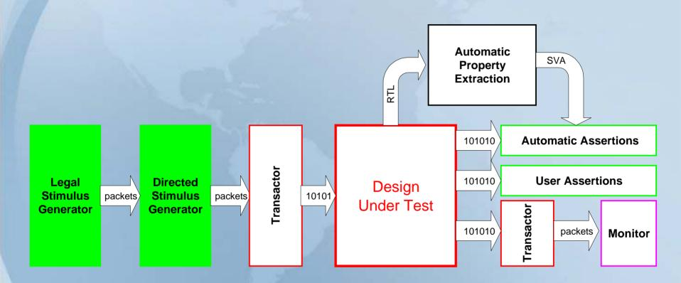
This is the complete simulation testbench
