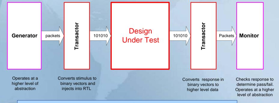
Modularized verification: Complete separation of stimulus generation and results checking enables reuse
