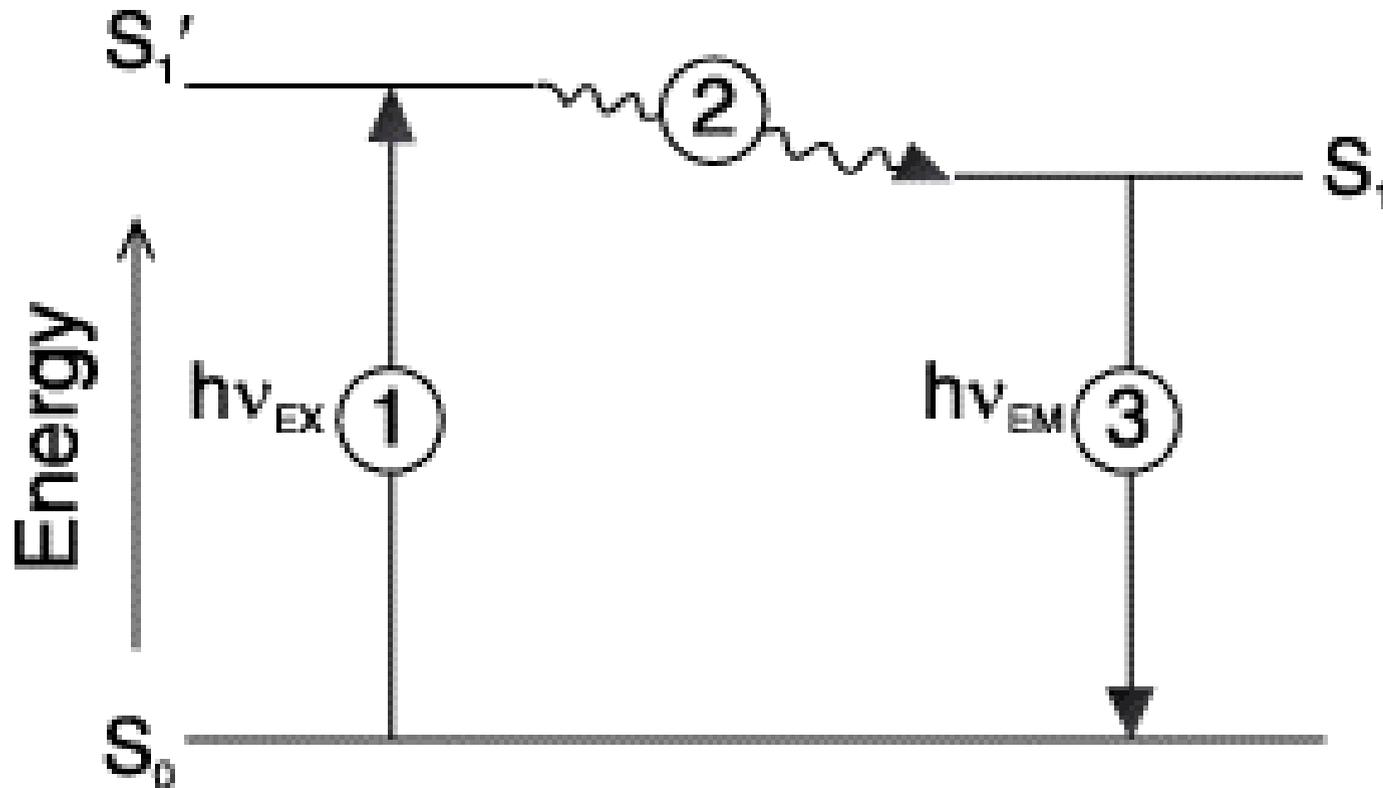
Jablonski diagram illustrating the processes involved in the creation of an excited electronic singlet state by optical absorption and subsequent emission of fluorescence.
