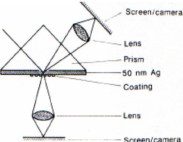
Fig. 1 Schematic of the optical set-up of SPM. Not to scale.
