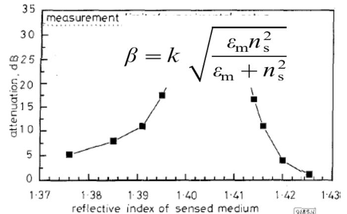
**Fig.1** Measured mode attenuation against refractive index of sensed medium
