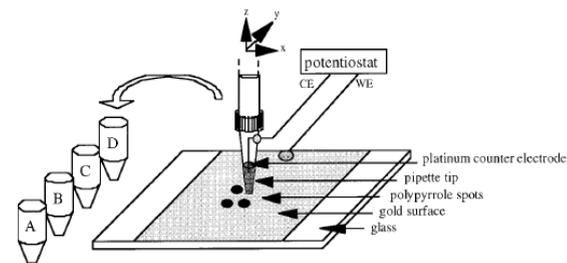
**Figure 1.** General scheme of the polypyrrole electrospotting methodology: The different tubes A–D containing different pyrrole–ODN and pyrrole monomer solutions are on the left. The spotting is carried out on the gold surface via the plastic tip containing the solution to be copolymerized.
