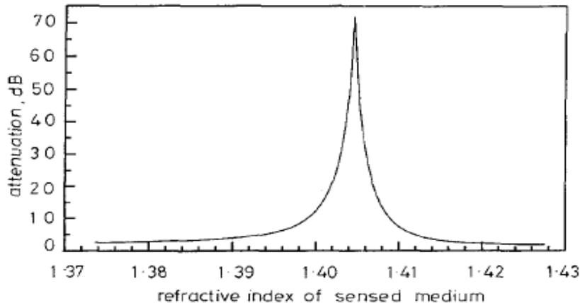
**Fig. 2** Dependence of fibre mode attenuation on refractive index of sensed medium
