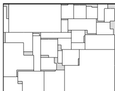
Figure 10: Resulting placement of ami49_LT (area = 37.37mm^2 ).
