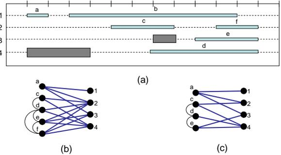
Figure 7: The process for track assignment. (a) The final track assignment for the instance of Figure 6. (b) The resulting combination graph after assigning  $b$  to track 1. (c) The resulting combination graph after assigning  $f$  to track 2.
