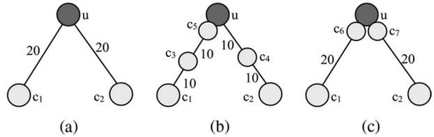
Fig. 4. (a) Routing tree with one sink node  $u_1$ . (b) Work in [10] needs jumpers  $c_3$ ,  $c_4$ , and  $c_5$  to solve the antenna violations. (c) This paper needs only two jumpers,  $c_6$  and  $c_7$ , to satisfy the antenna rule.
