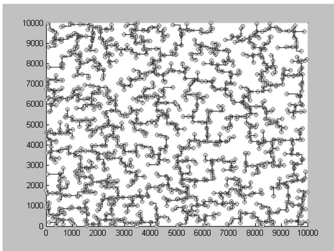
Fig. 17. Layout resulting from the BUJI algorithm with 429 jumpers for antenna fixing on a tree with 1615 nodes. Circles denote the nodes of the routing tree and the  $\times$  signs denote the inserted jumpers.
