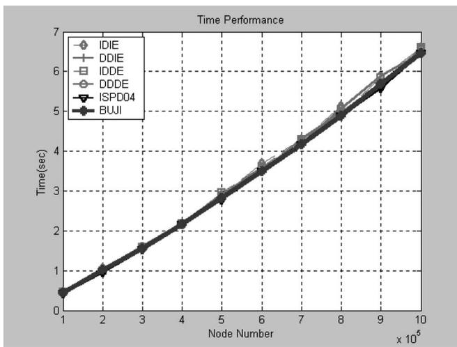
Fig. 16. CPU times required for antenna fixing for routing trees of various numbers of nodes.
