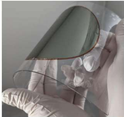
Fig. 3: Optical image of the Ge membrane transferred to flexible substrate using adhesive tape
