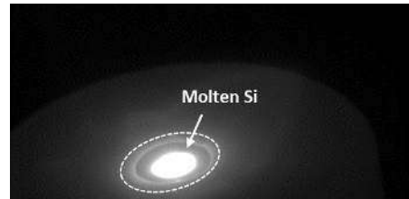
Fig. 2. Photograph of a cylindrical Si source (12 mm in diameter and 8 mm in height) during evaporation.
