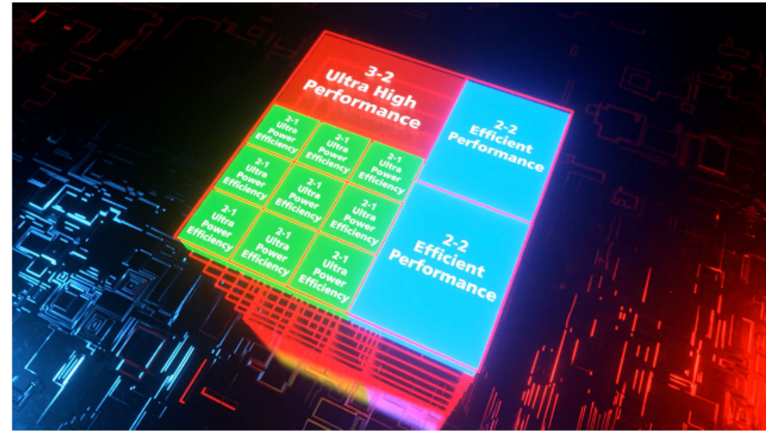
Diagram 2: N3 with FINFLEX enables a designer to choose the ideal FIN configuration for each functional block on a chip.
