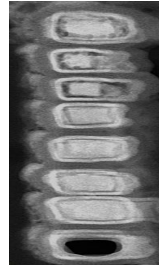
NTU 8 stacked nanosheets Chung-En Tsai et al. and C. W. Liu, International Electron Devices Meeting (IEDM), 2021.
